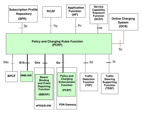
Figure E.3.4.1: Gx, Gxx and S15 reference point at the Policy and Charging Control (PCC) architecture with SPR
