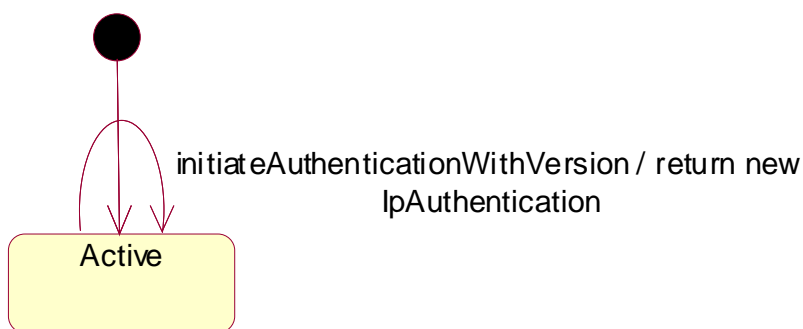
Figure : State Transition Diagram for IpInitial
