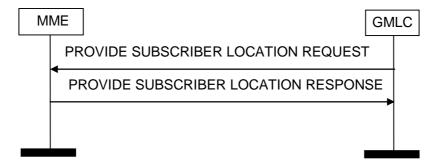
Figure 6.2.2-1: Provide Subscriber Location procedure. Successful operation.
