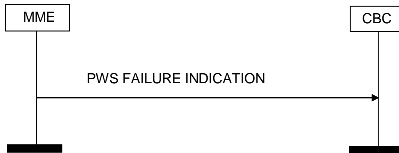
Figure 4.3.3F.2-1: PWS Failure Indication, Successful Operation.
