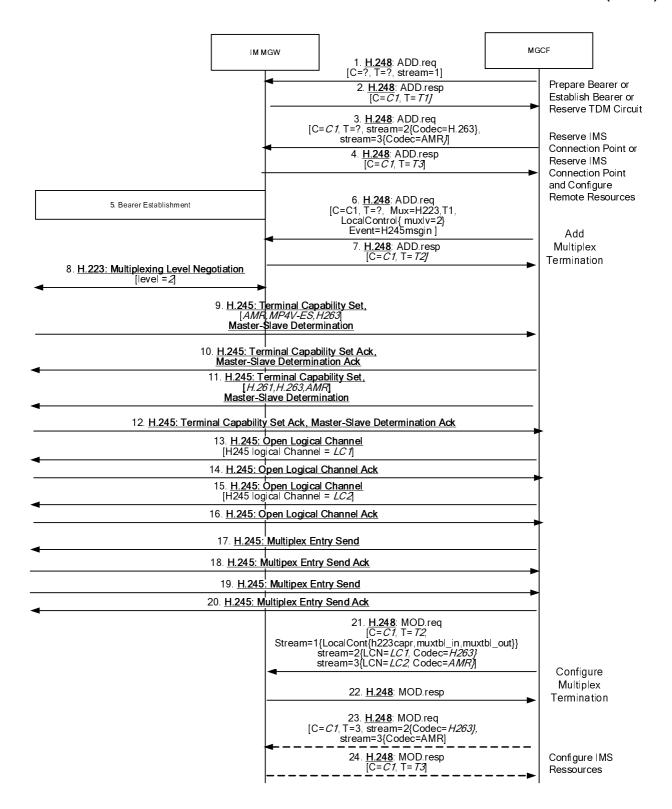
NOTE 1: All H.245 messages (from Signal 9 to Signal 18) are transported through the IM-MGW between the MGCF and the CS side, using the procedures described in subclause E.4.2.3
