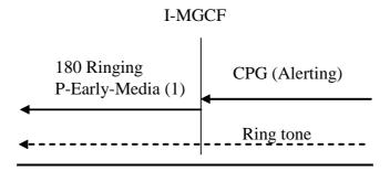
NOTE: The P-Early-Media header field is a included if the received INVITE contains a P-Early-Media header field with the "supported" parameter as described in IETF RFC 5009 [89].
