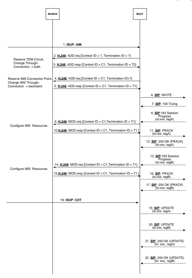
Figure 39a/1: CS Network Originating Session with forking, ISUP (message sequence chart)
