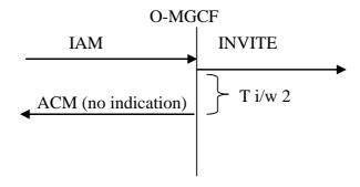
Figure 17: Sending of ACM (Ti/w<sub>2</sub> elapses)
