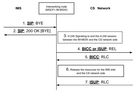
NOTE: Signal 7 is omitted when IM CN subsystem interworks with BICC based CS network and Signal 5 is omitted when IM CN subsystem interworks with ISUP based CS network.
