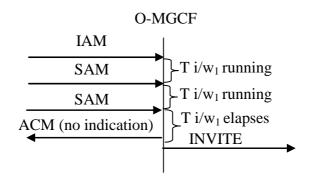
Figure 15: Sending of ACM T i/w<sub>1</sub> elapses
