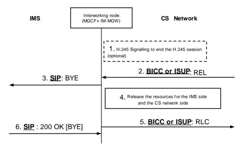
Figure E.2.6.2.1: Call release initiated from the CS network side
