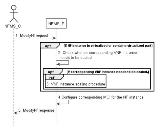
Figure 7.11-1: Network Function Instance Modify procedure
