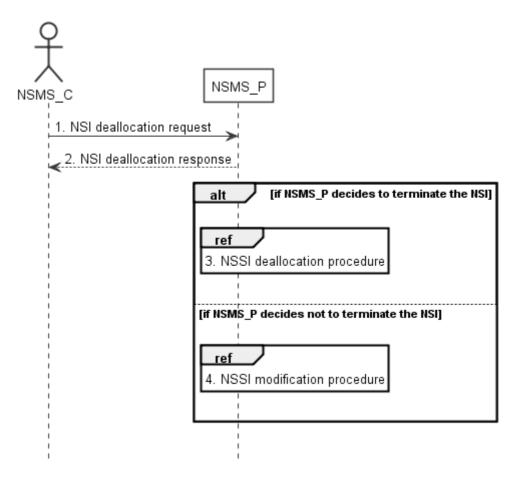
Figure 7.4-1: Network slice instance deallocation procedure
