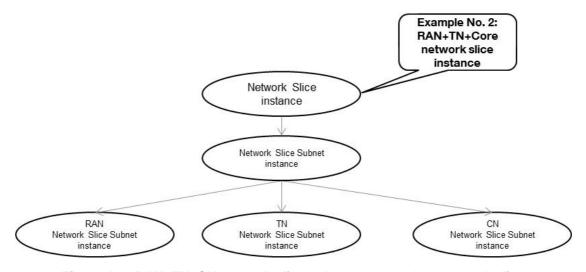
Figure A.4: RAN+TN+CN network slice subnets exposed as network slice
