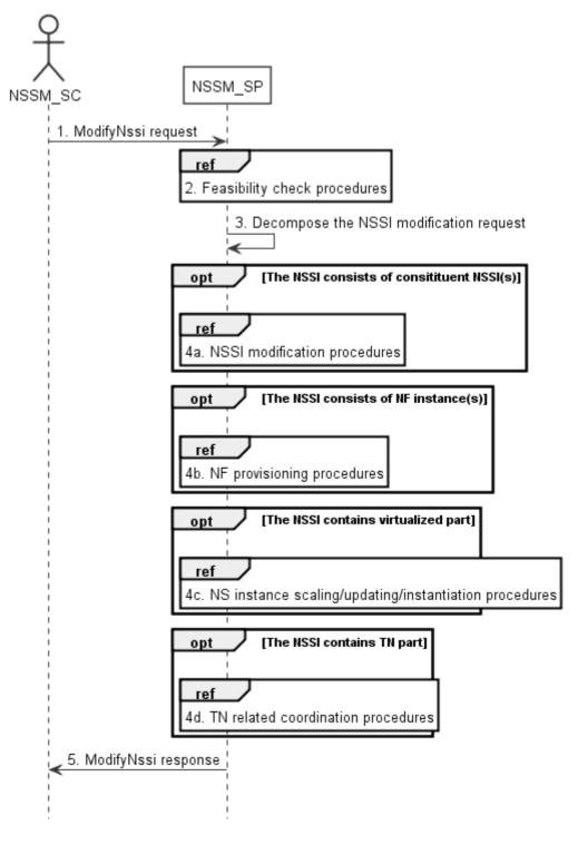
Figure 7.7-1: Network Slice Subnet Instance Modification Request procedure
