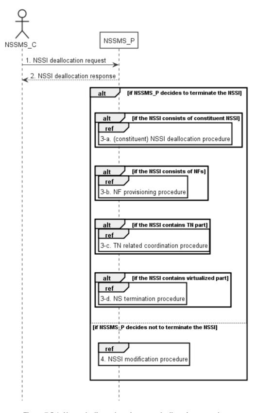
Figure 7.5-1: Network slice subnet instance deallocation procedure
