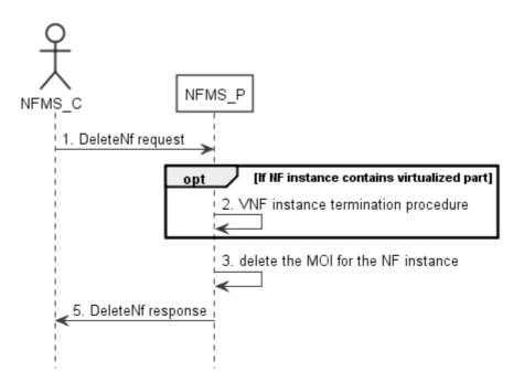
Figure 7.12-1: Network Function Instance Deletion procedure
