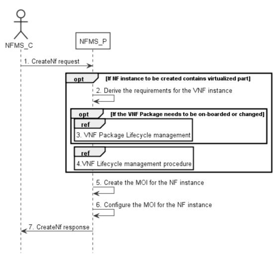
Figure 7.10-1: Network Function Instance Creation procedure
