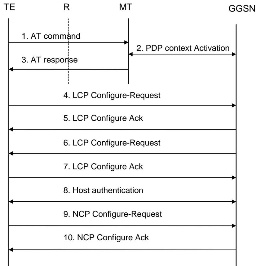
**Figure 9a: PPP Based Service (transparent PPP negotiation)**
