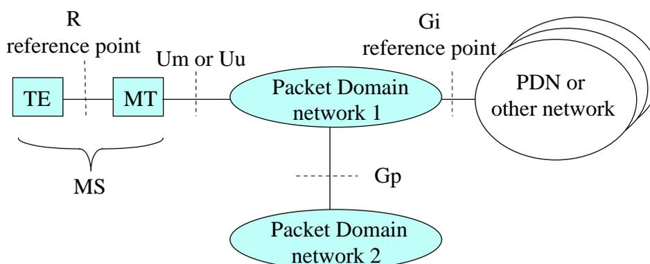
**Figure 1: Packet Domain Access Interfaces and Reference Points**
