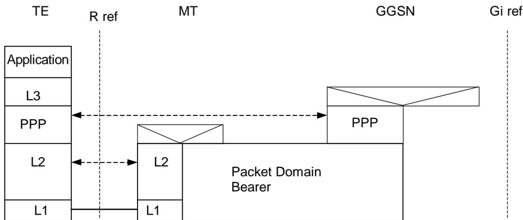
**Figure 8a: PPP Based Services (transparent PPP negotiation)**
