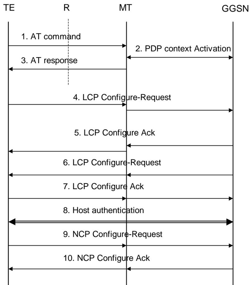
**Figure 9b: PPP Based Service (relayed PPP negotiation)**
