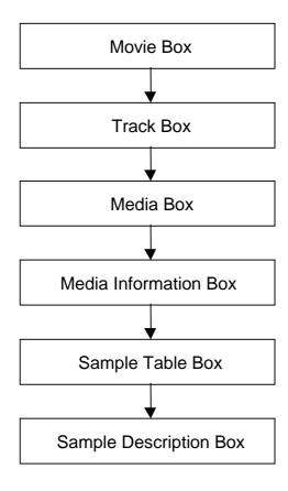
Figure 6.1: ISO File Format Box Structure Hierarchy
