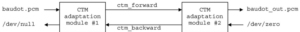
A CTM implementation and a Baudot 45.45 baud codec shall be combined to form a CTM adaptation module under test. The source code for an example implementation of this CTM adaptation module is provided in [2]. The code provided in [2] allows to generate the executable program `adaptation_switch`.
