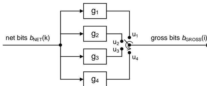
Figure 3 – Structure of the convolutional encoder
