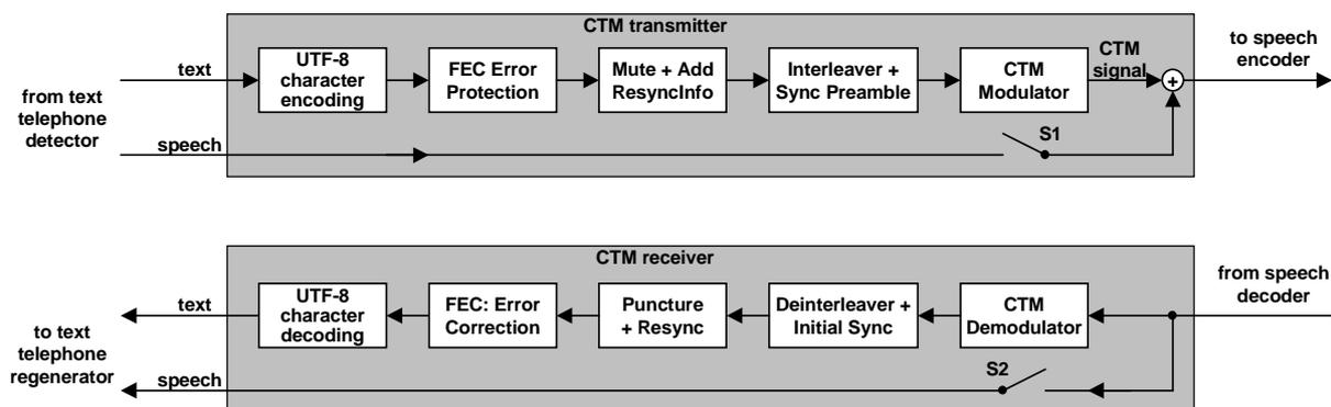
Figure 2 – Overview of the CTM Transmitter and Receiver
