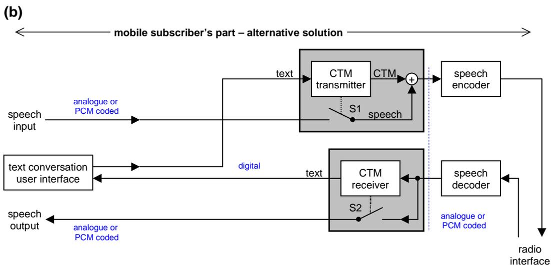
**Figure 1 – One Text Telephony architecture using CTM**
