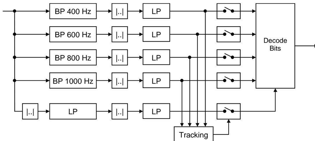
**Figure A.1 – Structure of the CTM demodulator**
