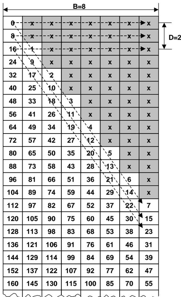
Figure 6 – Interleaver matrix and location of the preamble
