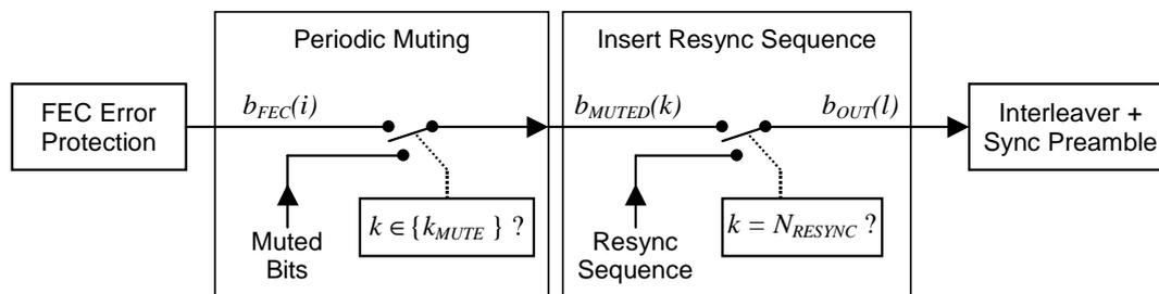
Figure 4 – Periodic muting and insertion of resynchronisation sequence
