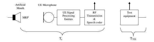
Figure 17b1: Different entities contributing to the delay in sending direction
