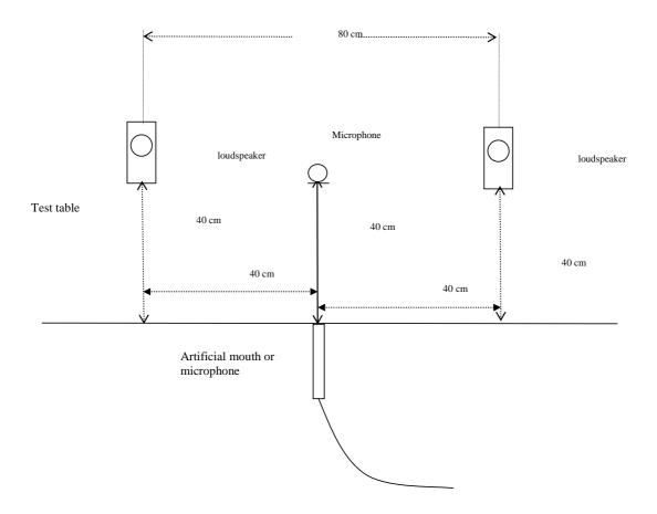
Figure 14: Configuration of a softphone using external speakers and a microphone relative to microphone or artificial mouth viewed from above
