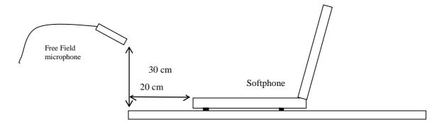
Figure 8: Configuration of a softphone relative to the free field microphone side view
