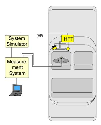
Figure 3a: Test Configuration for vehicle mounted hands-free, using HATS
