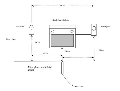
Figure 12: Configuration of a softphone using external speakers relative to microphone or artificial mouth viewed from above
