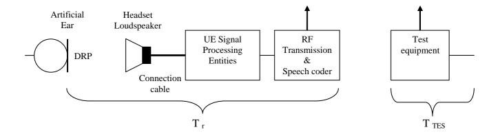
Figure 19b4: Different entities contributing to the delay in receiving direction with a headset connected via cable
