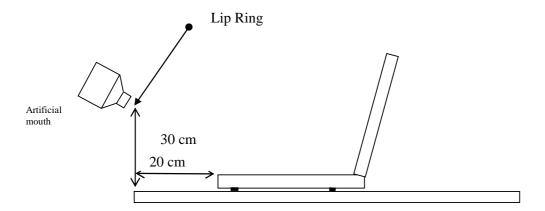
Figure 7: Configuration of a softphone relative to the artificial mouth side view
