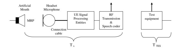
Figure 19b2: Different entities contributing to the delay in sending direction with a headset connected via cable
