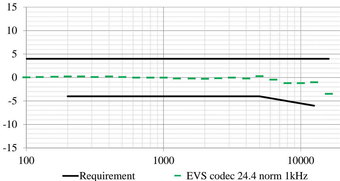
Figure 15: Handset and headset sending sensitivity/frequency masks. The frequency response of the EVS codec operating as specified in TS 26.132 (super-wideband 24,4kbit/s, using the specified P.501 speech test signal), is plotted for reference, normalized to 0dB at 1kHz.
