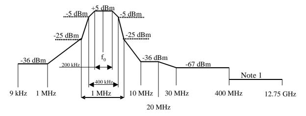
Figure 4.3.4.2.1: Modem spectrum emission mask.
