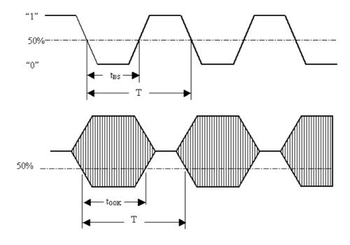
Duty cycle for bit stream =  $t_{BS}/T$ ; duty cycle for OOK =  $T_{OOK}/T$
