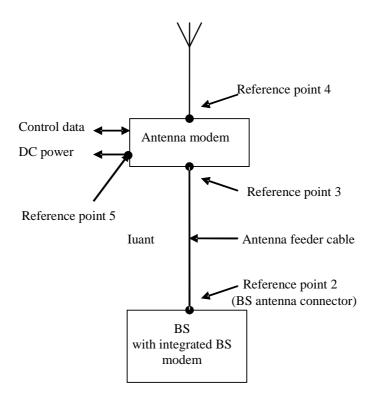
Figure 4.3.2: Modem configuration and modem reference points for a BS with integrated BS modem
