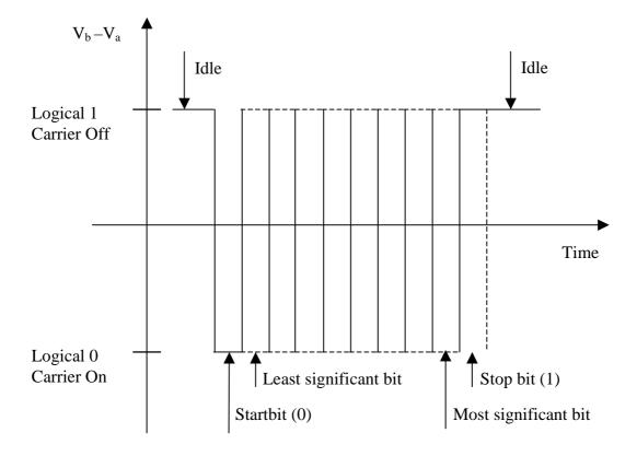
Figure 4.1.1: Format and order of transmitted data
