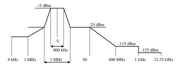
Figure 4.3.4.2.1: Modem spectrum emission mask.
