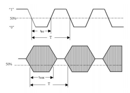
Duty cycle for bit stream = t<sub>BS</sub>/T; duty cycle for OOK = T<sub>OOB</sub>/T
