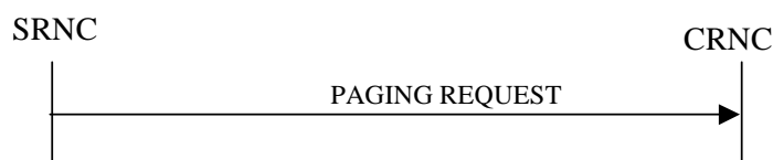
Figure 4: Paging procedure, Successful Operation
