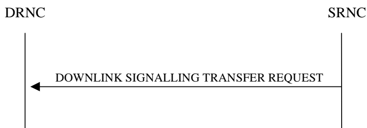
Figure 2: Downlink Signalling Transfer procedure, Successful Operation
