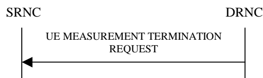
Figure 261: UE Measurement Termination procedure, Successful Operation
