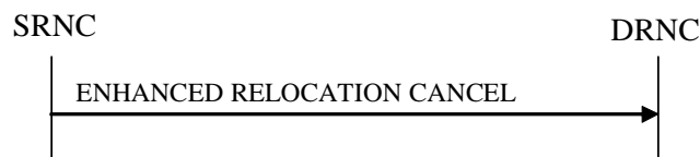
Figure 260: Enhanced Relocation Cancel procedure: Successful Operation
