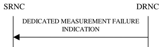
Figure 24: Dedicated Measurement Failure procedure, Successful Operation
