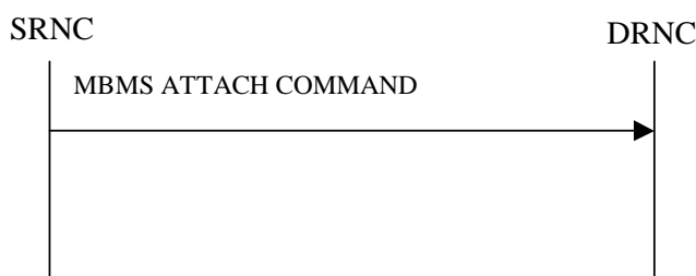
Figure 31: MBMS Attach procedure, Successful Operation
