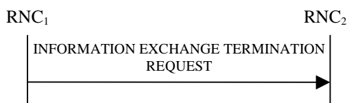
Figure 30I: Information Exchange Termination procedure, Successful Operation
