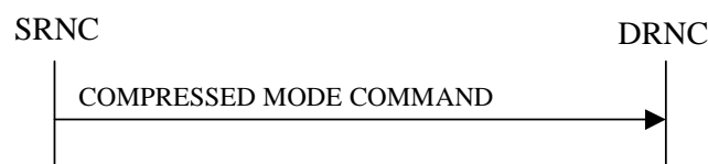
Figure 26: Compressed Mode Command procedure, Successful Operation
