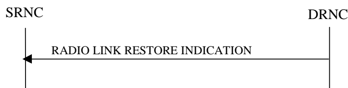
Figure 19: Radio Link Restoration procedure, Successful Operation
