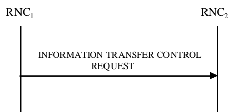
Figure 30M: Information Transfer Control procedure, Successful Operation
