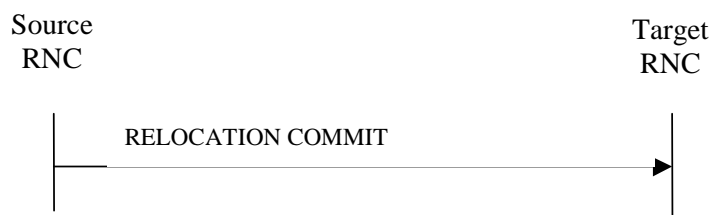
Figure 3: Relocation Commit procedure, Successful Operation
