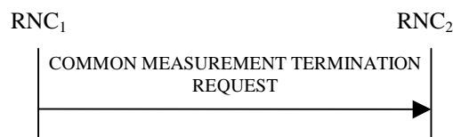
Figure 30D: Common Measurement Termination procedure, Successful Operation
