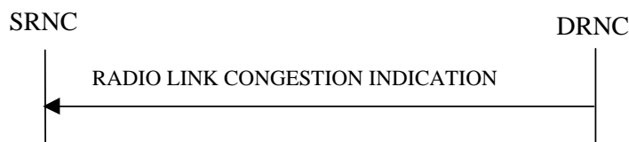
Figure 26C: Radio Link Congestion procedure, Successful Operation
