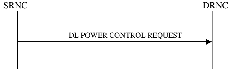
Figure 25: Downlink Power Control procedure, Successful Operation
