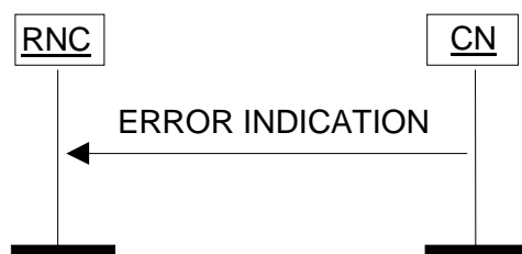
Figure 31: Error Indication procedure, CN originated. Successful operation.
