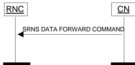
Figure 13: SRNS Data Forwarding Initiation procedure. Successful operation.
