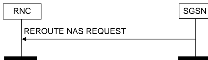
Figure 64: Reroute NAS Request procedure: Successful operation.
