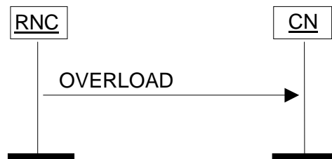
Figure 28: Overload at the UTRAN. Successful operation.
