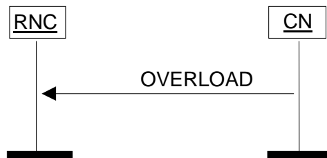
Figure 27: Overload at the CN. Successful operation.
