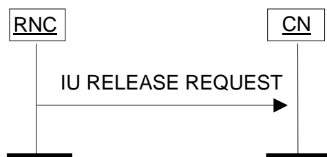
Figure 3: Iu Release Request procedure. Successful operation.
