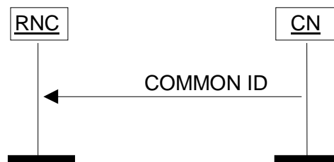
Figure 17: Common ID procedure. Successful operation.
