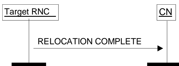
Figure 10: Relocation Complete procedure. Successful operation.
