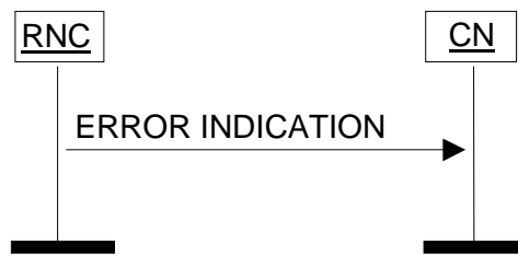
Figure 32: Error Indication procedure, RNC originated. Successful operation.
