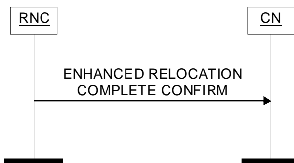
Figure 60: Enhanced Relocation Complete Confirm procedure. Successful operation.
