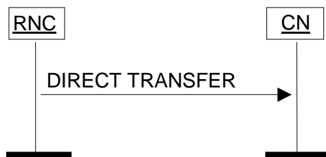
Figure 26: Direct Transfer, RNC originated. Successful operation.
