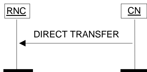
Figure 25: Direct Transfer, CN originated. Successful operation.
