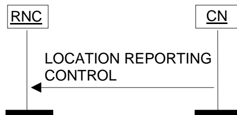
Figure 21: Location Reporting Control procedure. Successful operation.
