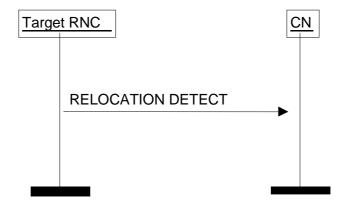
Figure 9: Relocation Detect procedure: Successful operation.
