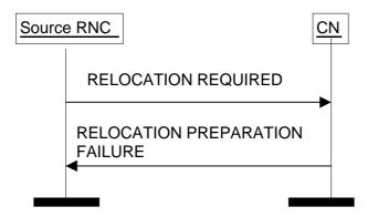
Figure 6: Relocation Preparation procedure. Unsuccessful operation.
