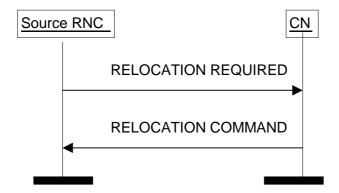
Figure 5: Relocation Preparation procedure. Successful operation.
