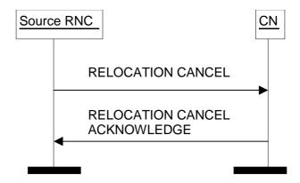
Figure 11: Relocation Cancel procedure. Successful operation.
