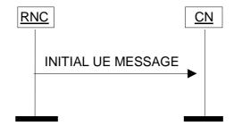
Figure 24: Initial UE Message procedure. Successful operation.
