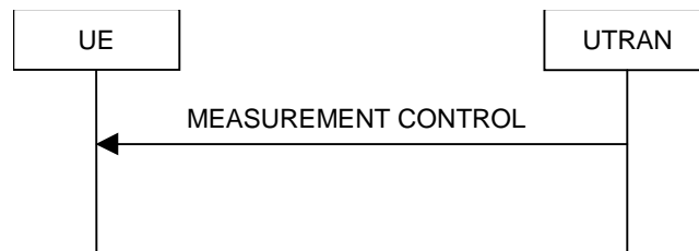
Figure 8.4.1-1: Measurement Control, normal case
