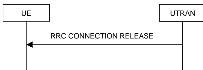
Figure 8.1.4-2: RRC Connection Release procedure on the CCCH
