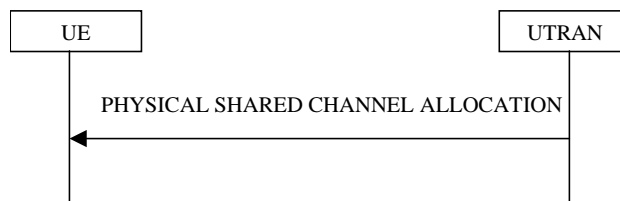
Figure 8.2.7-1: Physical Shared Channel Allocation
