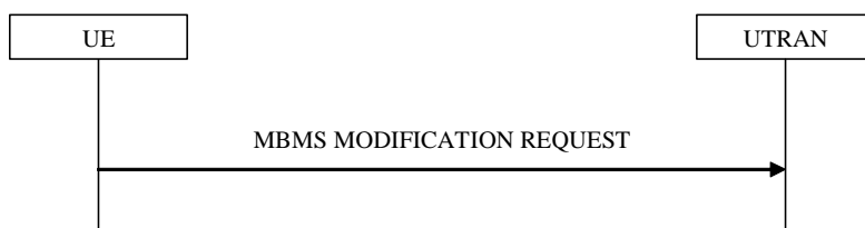
Figure 8.7.6-1: MBMS modification request, normal
