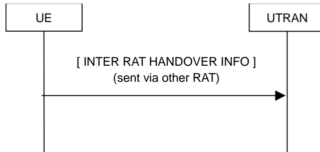
Figure 8.1.16-1: Inter RAT handover information transfer, normal flow
