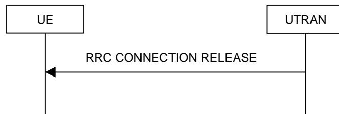
Figure 8.1.4-2: RRC Connection Release procedure on the CCCH
