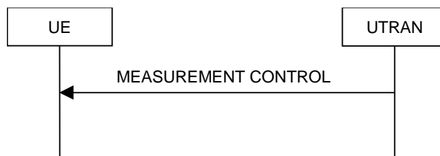
Figure 8.4.1-1: Measurement Control, normal case
