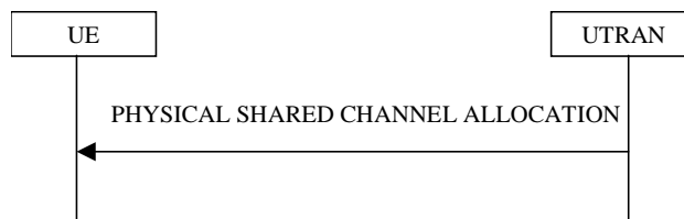
Figure 8.2.7-1: Physical Shared Channel Allocation
