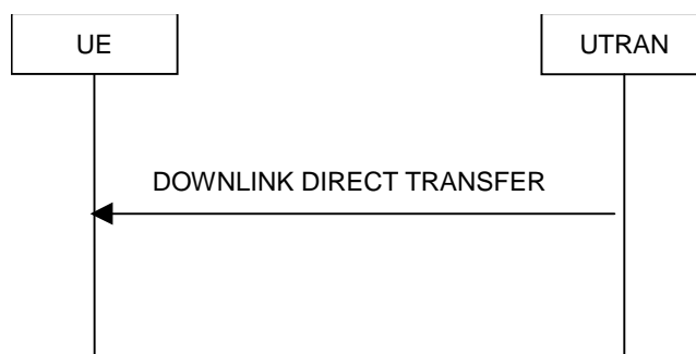
Figure 8.1.9-1: Downlink Direct transfer, normal flow
