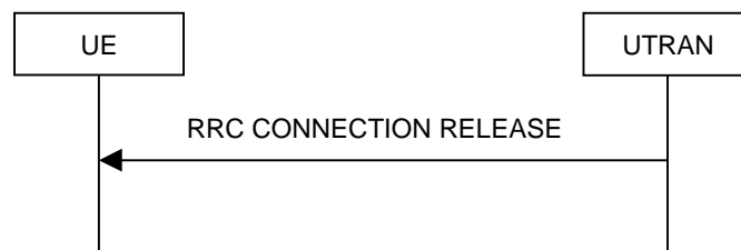
Figure 8.1.4-2: RRC Connection Release procedure on the CCCH
