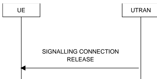
Figure 8.1.13-1: Signalling connection release procedure, normal case
