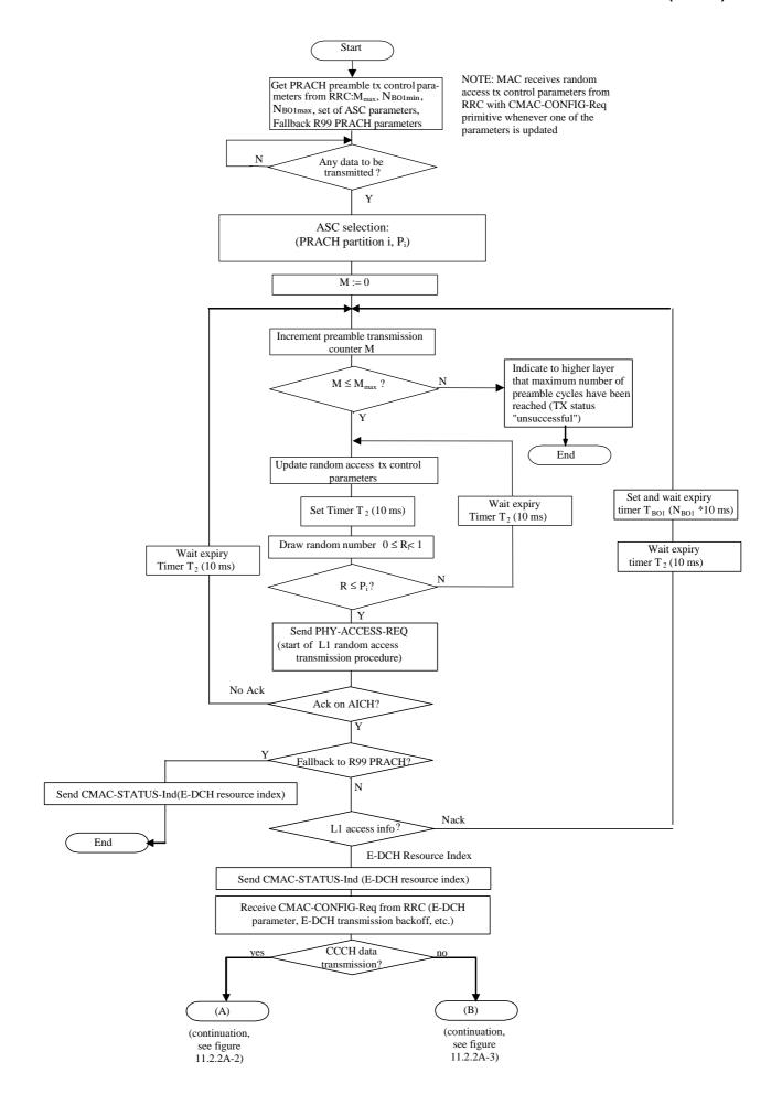
Figure 11.2.2A-1: Enhanced Uplink in CELL\_FACH state and Idle mode transmission control procedure (UE side, informative) with Fallback to R99 PRACH, Part I
