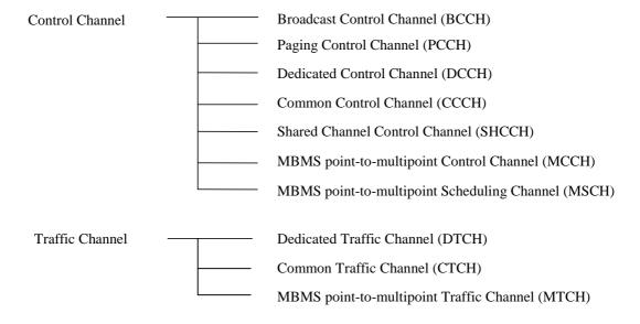
Figure 4.3.2.1-1: Logical channel structure
