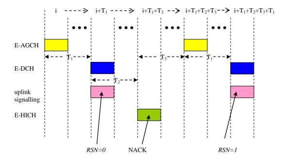
Figure 11.9.1.1-1: TDD E-DCH HARQ Operation
