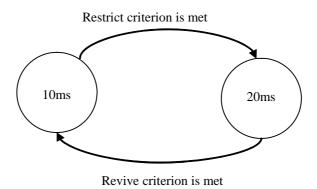
Figure 11.4.1-1: Transmission Mode Switching transitions for a given TFC
