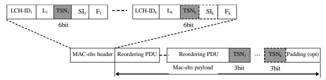
Figure 9.1.4-4: MAC-ehs PDU (1.28Mcps TDD multi-frequency HS-DSCH operation mode only)
