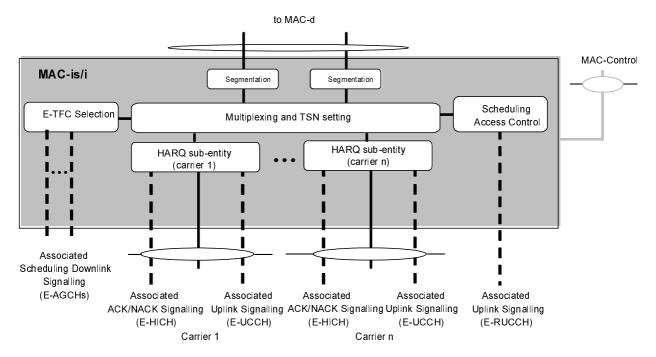
Figure 4.2.3.6-2a: UE side MAC architecture/MAC-i/is details (1.28Mcps TDD multi-carrier E-DCH carrier is configured)
