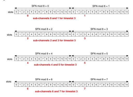
Figure 11.2.3.1-1 Eight sub-channels for timeslot 3
