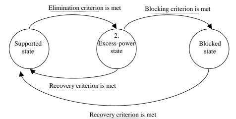
Figure 11.4-1: State transitions for the state of a given TFC
