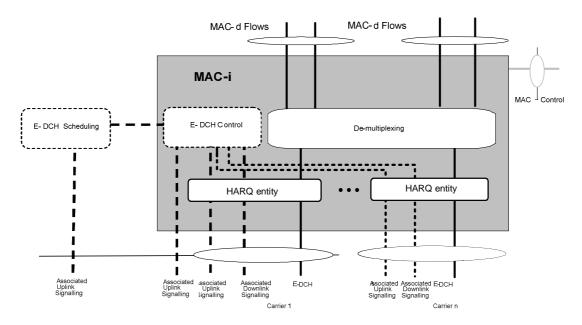
Figure 4.2.4.8-2a: UTRAN side MAC architecture / MAC-i details for muliti-carrier E-DCH operation (for 1.28Mcps TDD)
