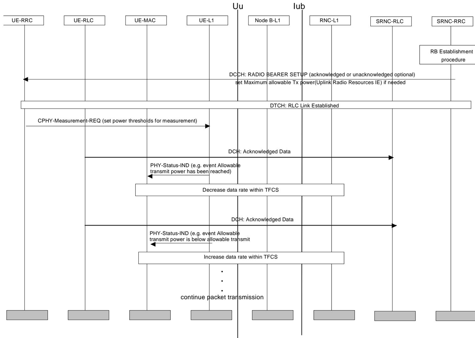
Figure 18: Variable Rate Transmission of Uplink DCHs
