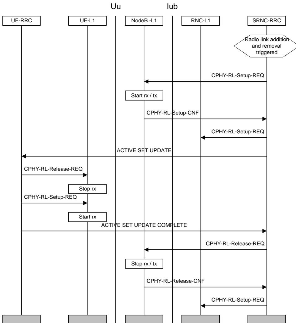
**Figure 32: Combined Radio Link Addition And Removal**
