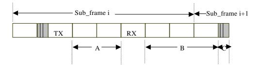
Figure A.2: Possible idle periods in a subframe with two occupied timeslots
