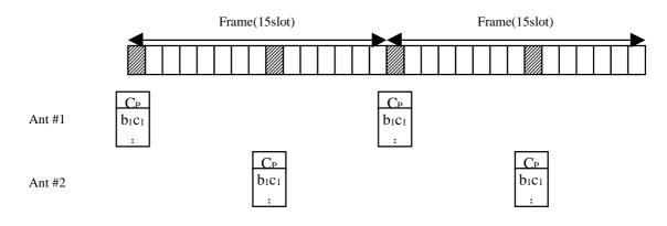
Figure 3: Antenna Switching Pattern (Case 2)
