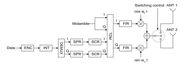
Figure 6: Example for TSTD Transmitter structure for DPCH/PDSCH and P-CCPCH.
