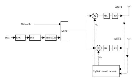
Figure 1: Downlink transmitter structure to support Transmit Diversity for PDSCH, DPCH, HS-SCCH, HS-PDSCH and E-AGCH transmission (UTRAN Access Point)
