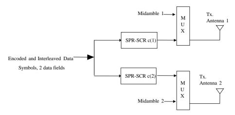
Figure 12: Block Diagram of the transmitter SCTD
