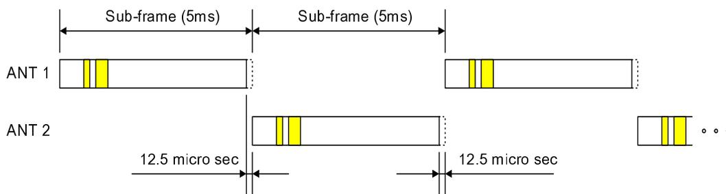
Figure 7: Example for the antenna swithing pattern for TSTD transmission of DPCH/PDSCH and P-CCPCH: all physical channels are transmitted with TSTD and are using the same antenna in the sub-frame.
