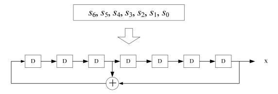
Figure 27: Structure of PN register
