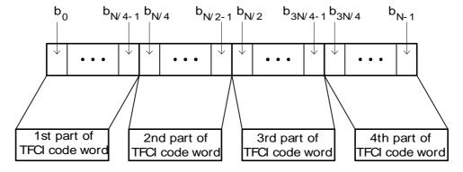
Figure 9: Mapping of TFCI code word bits to TFCI position in 1.28 Mcps TDD option, where N = N<sub>TFCI code word</sub>.
