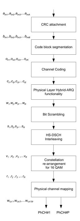
Figure 15: Coding chain for HS-DSCH
