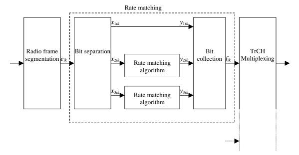
Figure 4: Puncturing of turbo encoded TrCHs
