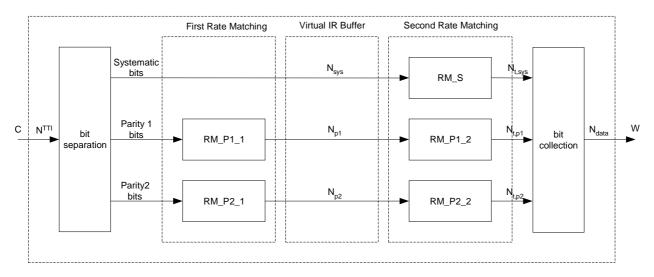
Figure 16: HS-DSCH hybrid ARQ functionality
