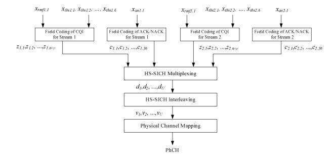
Figure 20A: Coding and multiplexing for HS-SICH type 2
