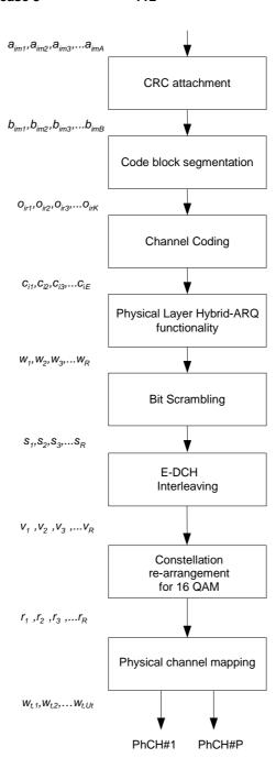
Figure 22. Coding chain for E-DCH
