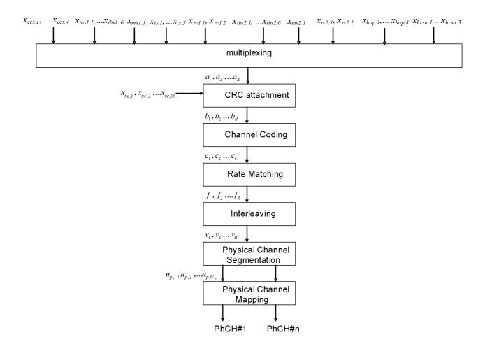
Figure 19H: Coding and Multiplexing for HS-SCCH type 9
