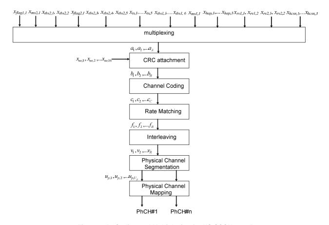
Figure 19D: Coding and Multiplexing for HS-SCCH type 5
