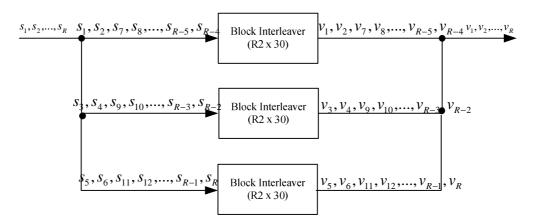
Figure 18a: Interleaver structure for HS-DSCH with 64-QAM modulation
