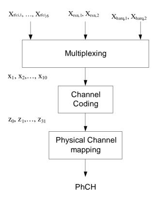
Figure 24A: Coding chain for E-UCCH
