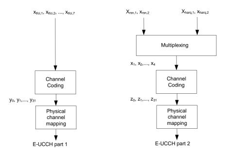
Figure 24: Coding chain for E-UCCH parts 1 and 2
