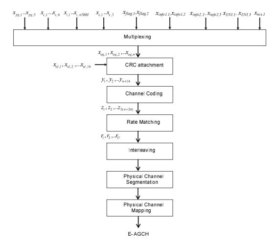
Figure 25A- TrCH processing of E-AGCH type2
