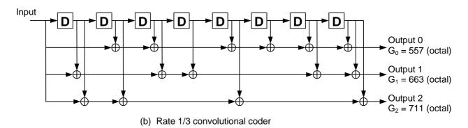
Figure 2: Rate 1/2 and rate 1/3 convolutional coders
