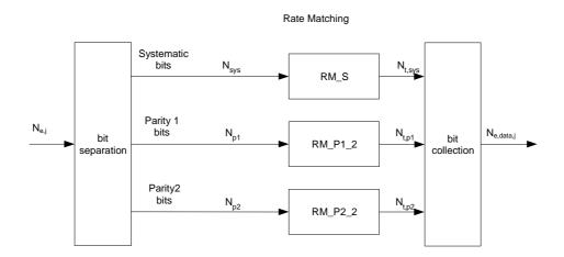
Figure 23: E-DCH hybrid ARQ functionality
