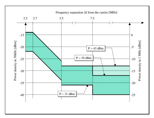
Figure 9.1: Illustrative diagram of spectrum emission mask
