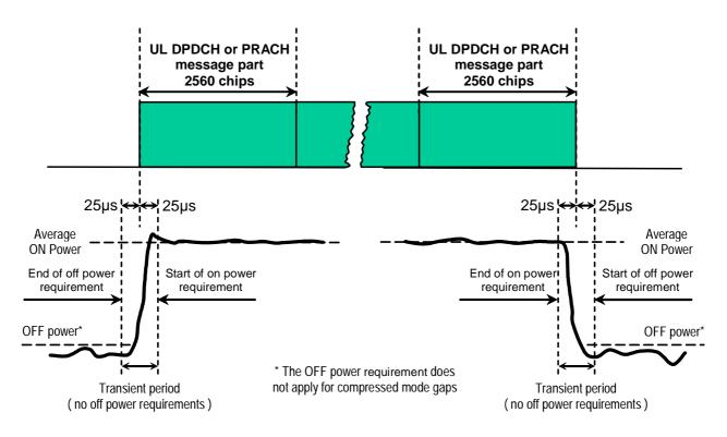
Figure 6.3: Transmit ON/OFF template for all other On/Off cases
