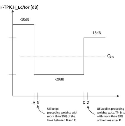
Figure 6.1C: Test case for F-TPICH out-of-quality handling in the UE supporting the optional enhanced requirements type1 for F-TPICH
