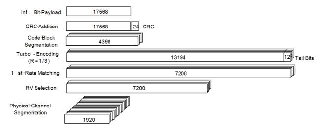
Figure A.29: Coding rate for Fixed Reference Channel H-Set 13 Primary and Fourth Transport Block
