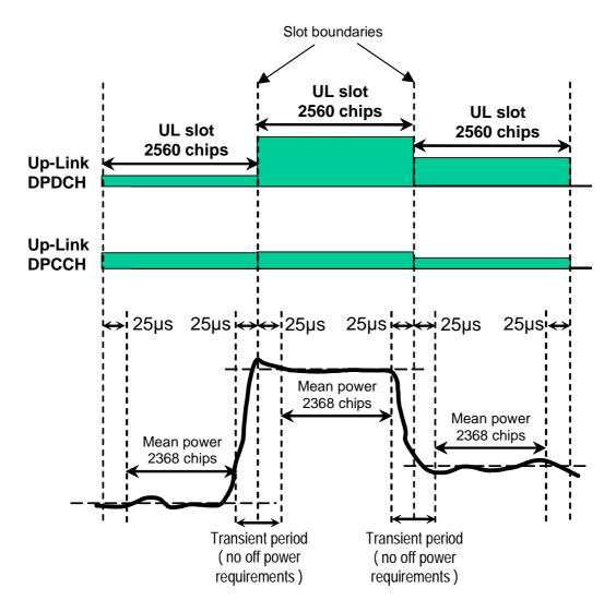
Figure 6.4: Transmit template during TFC change
