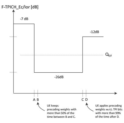
Figure 6.1B: Test case for F-TPICH out-of-quality handling in the UE supporting the minimum requirements for F-TPICH
