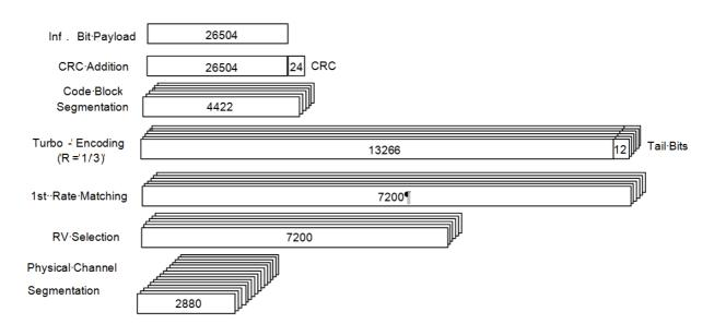
Figure A.31: Coding rate for Fixed Reference Channel H-Set 14 Primary and Fourth Transport Block
