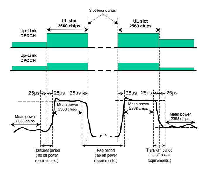
Figure 6.5: Transmit template during compressed mode
