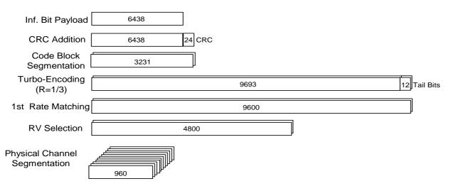
Figure A.20: Coding rate for Fixed reference Channel H-Set 6 (QPSK)
