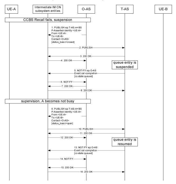
Figure A.2.1: CCBS suspend and resume procedures
