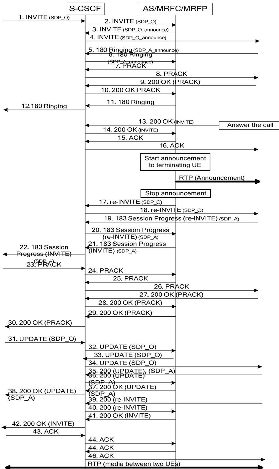
**Figure A.12: Announcement provided to the terminating UE when the called user answers the call and prior to establishing media stream between end users**
