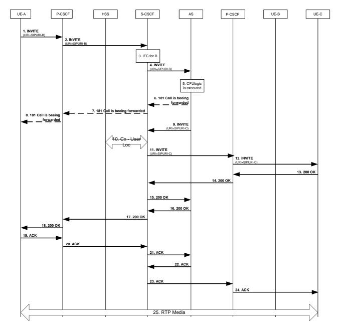
Figure A.1: CFU AS based normal case
