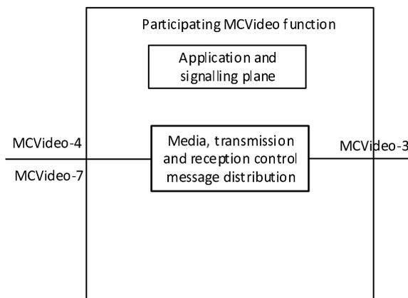
NOTE: The real internal structure of the participating MCVideo function is implementation specific but a possible internal structure is shown to illustrate the logic and the procedures.
