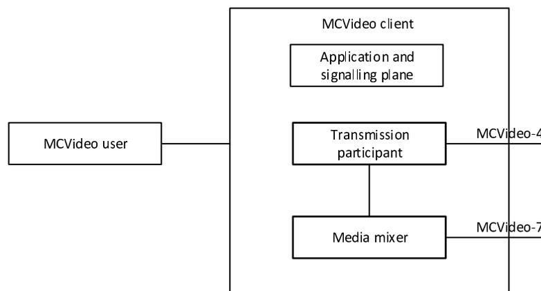
NOTE: The real internal structure of the MCVideo client is implementation specific but a possible internal structure is shown to illustrate the logic and the procedures.
