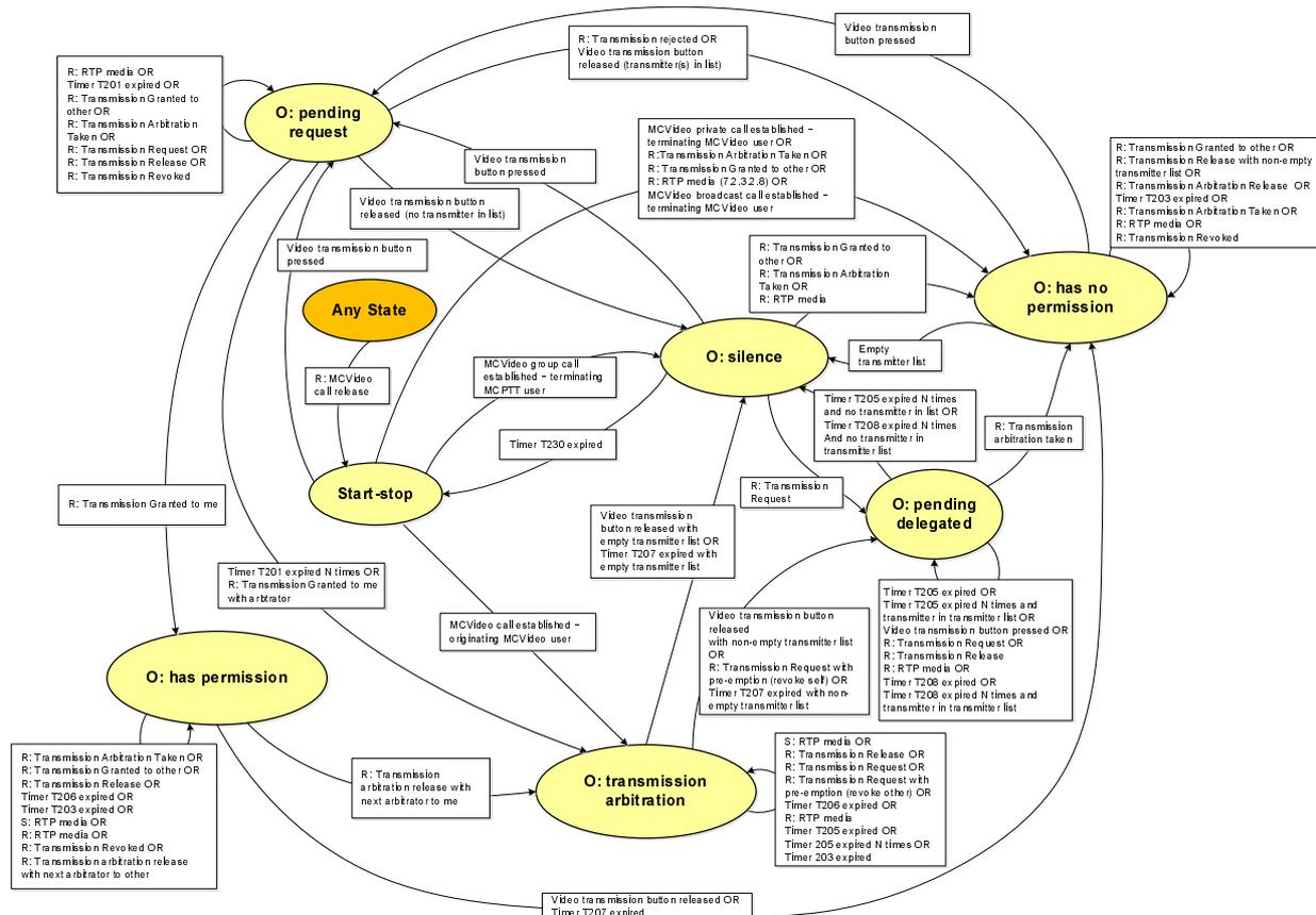
Figure 7.2.3.1-1: 'Transmission participant state diagram – basic operation'
