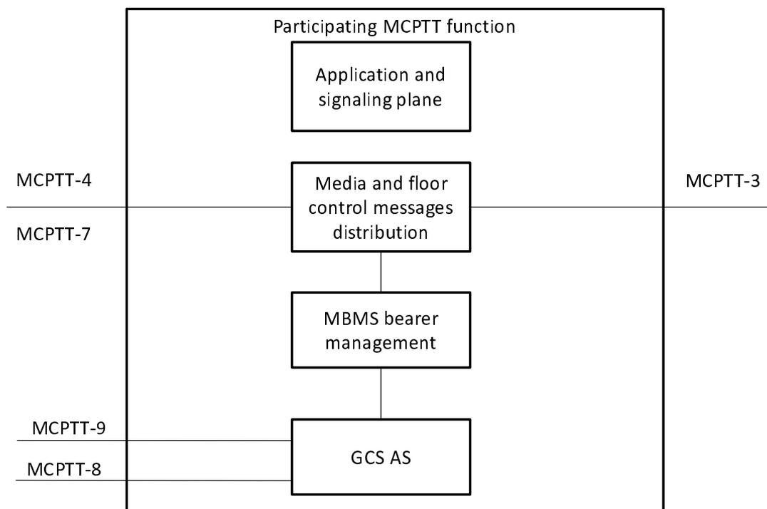
NOTE: The real internal structure of the participating MCPTT function is implementation specific but a possible internal structure is shown to illustrate the logic and the procedures.
