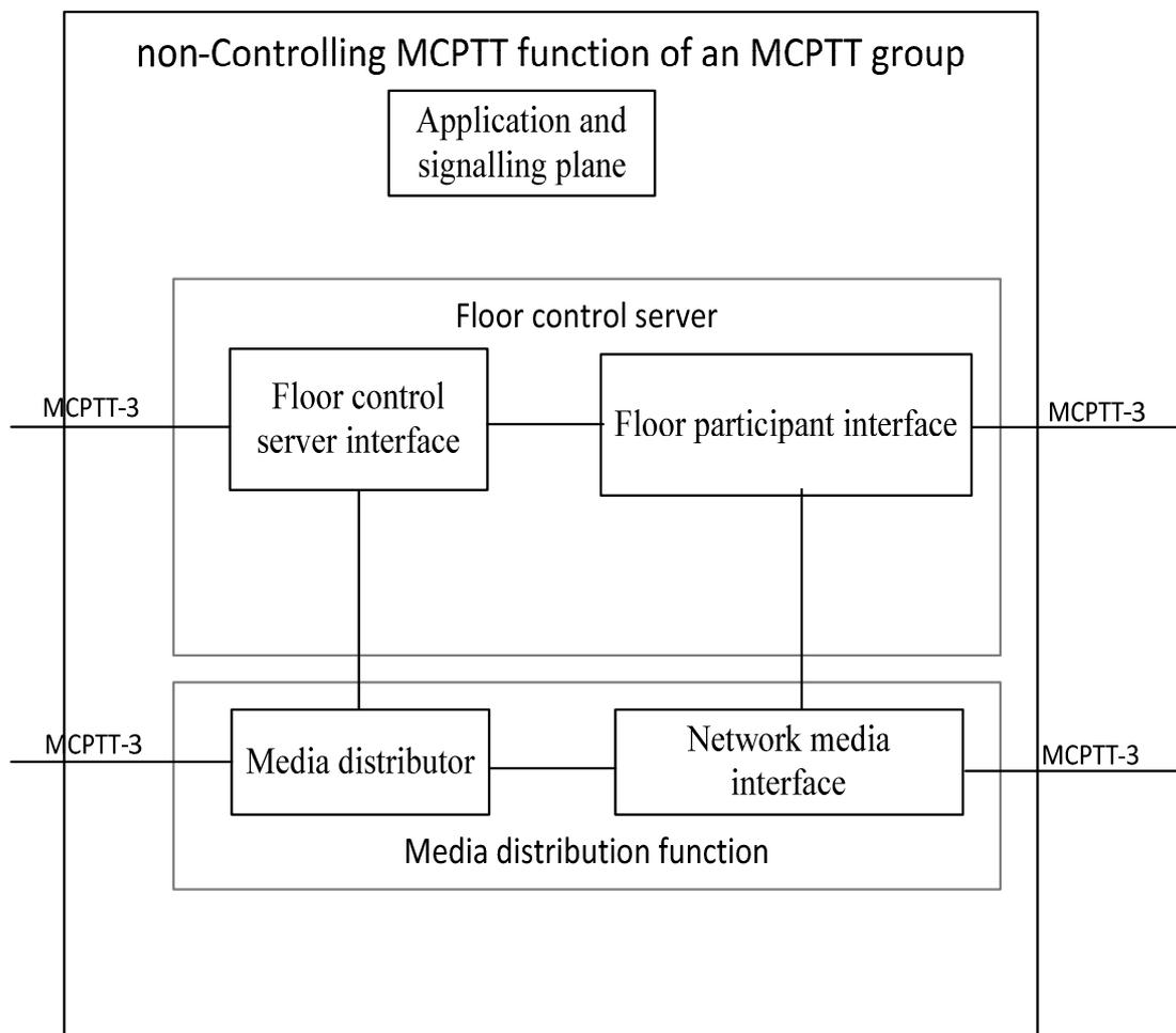
NOTE: The real internal structure of the MCPTT server is implementation specific but a possible internal structure is shown to illustrate the logic and the procedures.
