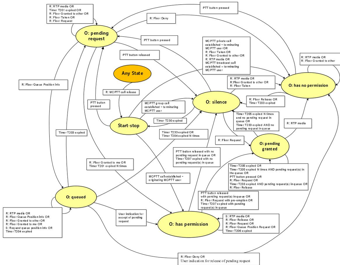
Figure 7.2.3.1-1: 'Floor participant state diagram – basic operation'
