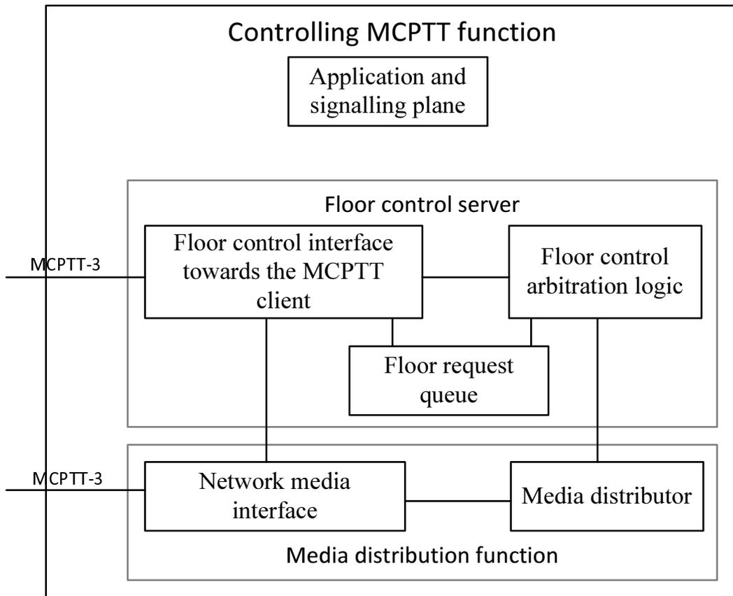
NOTE: The real internal structure of the MCPTT server is implementation specific but a possible internal structure is shown to illustrate the procedures.
