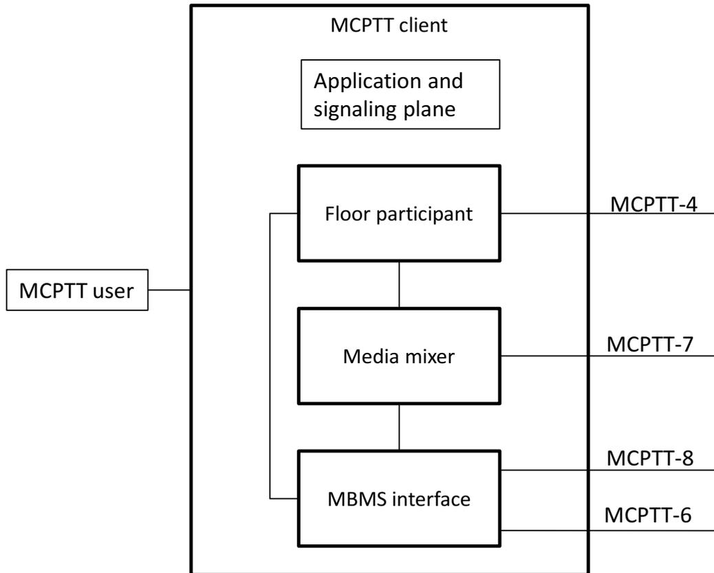
NOTE: The real internal structure of the MCPTT client is implementation specific but a possible internal structure is shown to illustrate the logic and the procedures.
