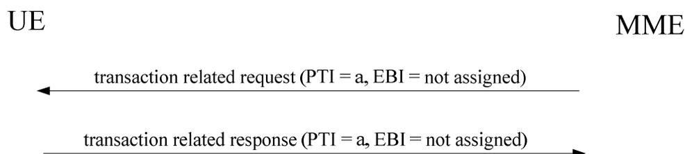
**Figure 6.3.2.2: Transaction related procedure initiated by the network**
