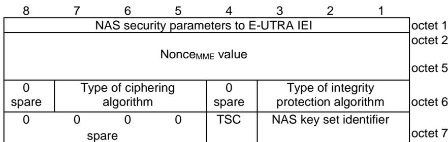
**Figure 9.9.2.7.1: NAS security parameters to E-UTRA information element**
