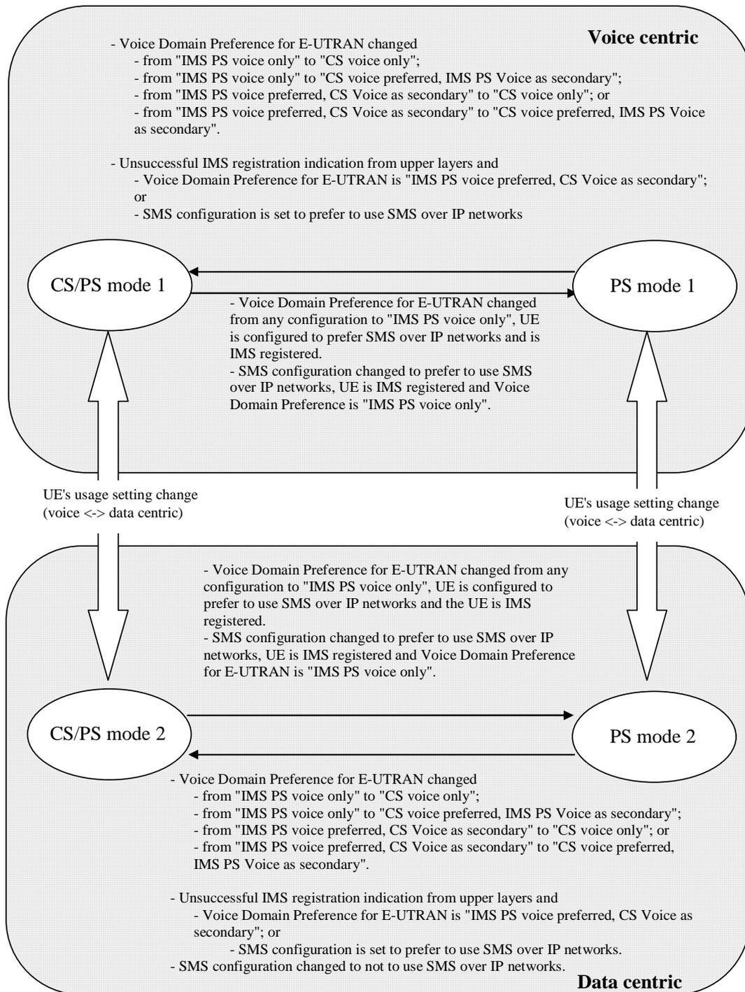
NOTE 1: The UE may transit from CS/PS mode 1 to PS mode 1 or from CS/PS mode 2 to PS mode 2 if "CS domain not available" is received. After the transition to PS mode 1 or PS mode 2 due to "CS domain not available", the UE can transit back to CS/PS mode 1 or CS/PS mode 2, e.g. due to change of PLMN which is not in the list of the equivalent PLMNs.
