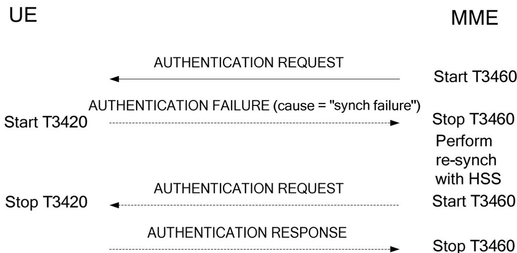
**Figure 5.4.2.7.2: Authentication failure procedure (EMM cause #21 "synch failure")**
