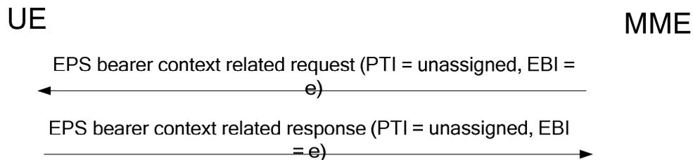
**Figure 6.3.2.4: EPS bearer context related procedure triggered network-internally**
