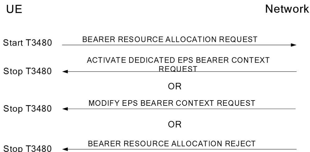
Figure 6.5.3.2.1: UE requested bearer resource allocation procedure
