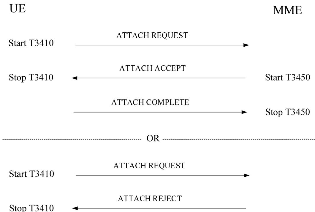
**Figure 5.5.1.2.2.1: Attach procedure and combined attach procedure**
