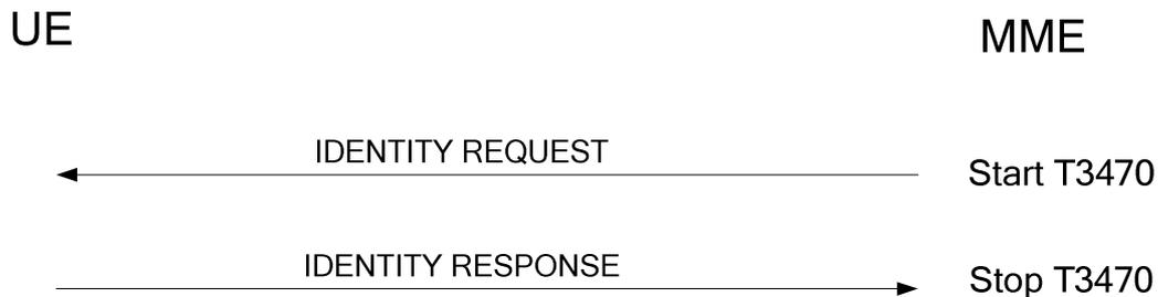
**Figure 5.4.4.2.1: Identification procedure**
