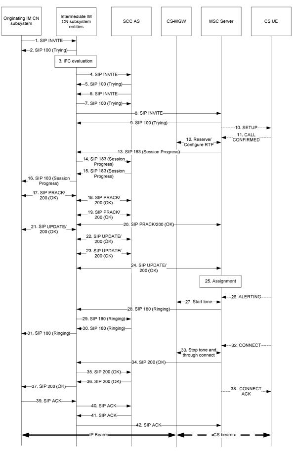
Figure A.5.1-1: CS UE Termination with CS media using an MSC Server enhanced for ICS (with codec negotiation)
