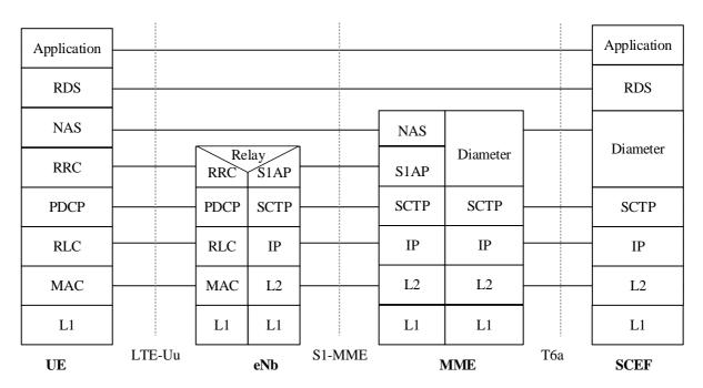
Figure 4.2-1: Protocol layering for reliable data transfer between UE and SCEF via E-UTRAN
