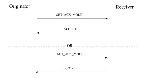
Figure 6.2.2.2-1: Establishment of acknowledged transfer procedure
