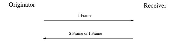
Figure 6.2.3.2-1: Acknowledged information transfer procedure
