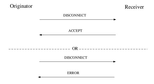
Figure 6.2.4.2-1: Termination of acknowledged transfer procedure
