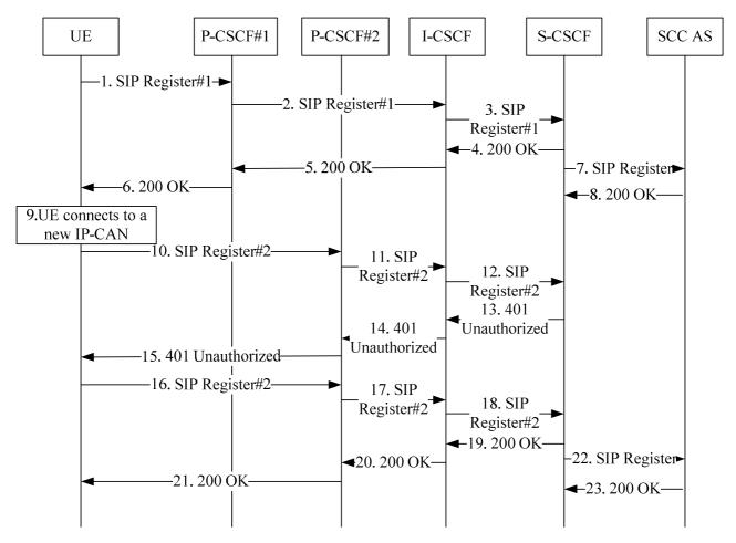
Figure A.3.2-1 Signalling flows for multiple registrations
