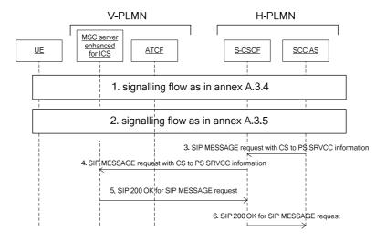
Figure A.3.6-1 registration with SRVCC enhancements
