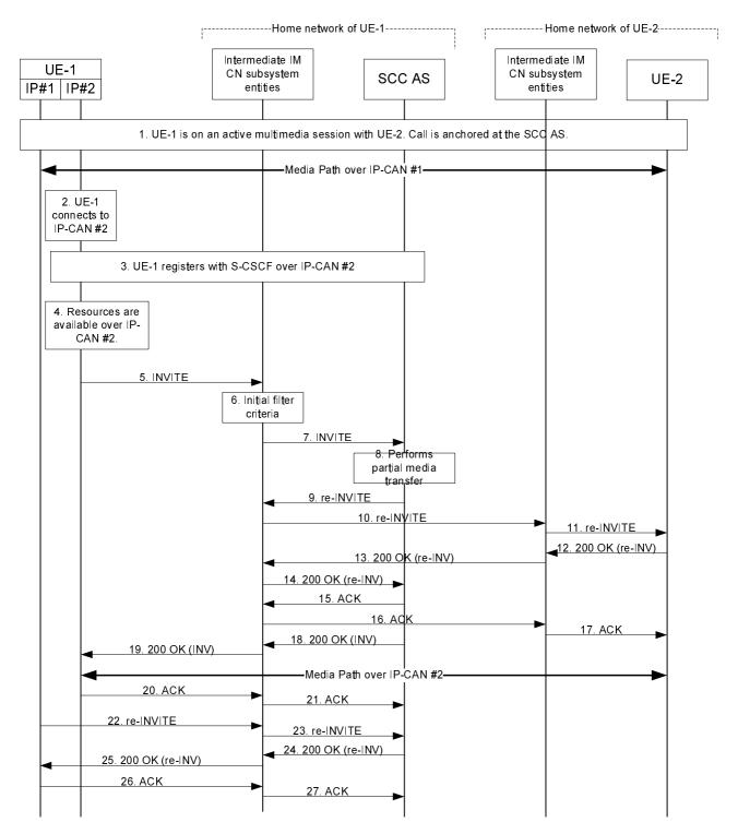
Figure A.7.3-1: Signalling flow for PS-PS session transfer with partial media transfer
