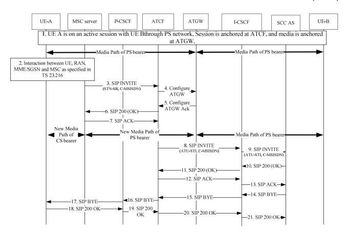
Figure A.18.3-1 Signalling flows for PS to CS access transfer: PS to CS SRVCC enhancements using ATCF and media anchored
