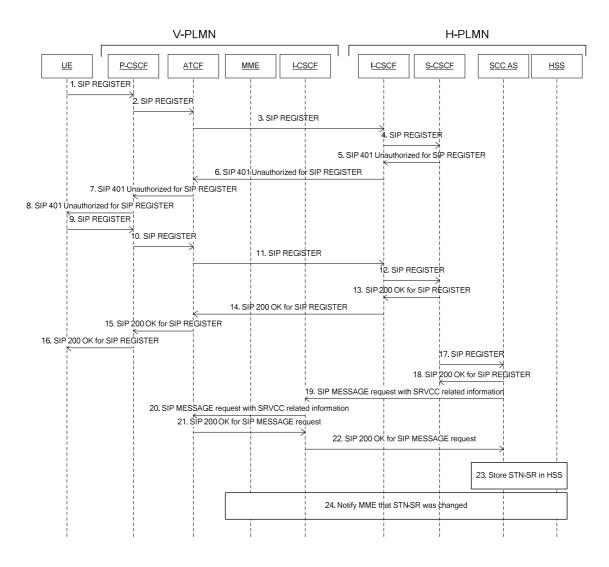
Figure A.3.3-1 registration with SRVCC enhancements
