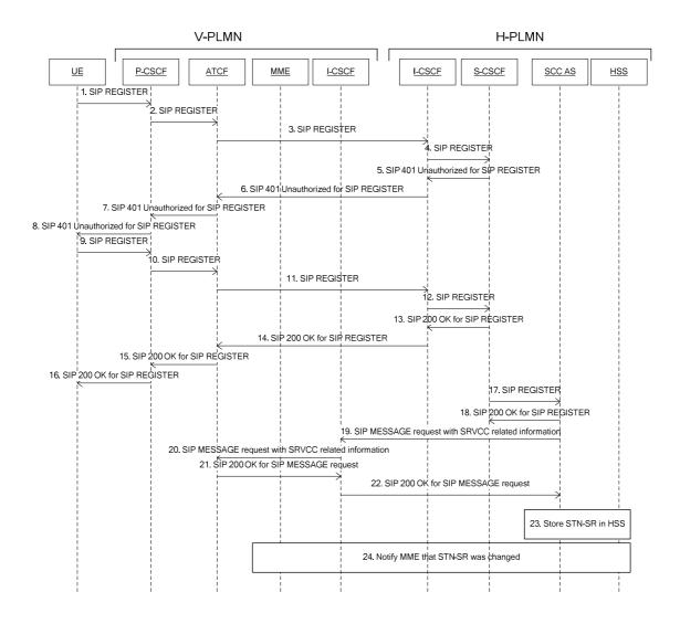
Figure A.3.3-1 registration with SRVCC enhancements
