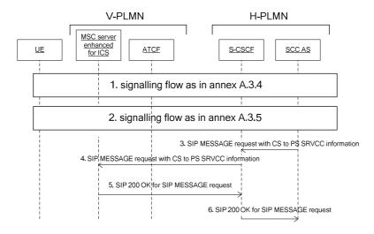
Figure A.3.6-1 registration with SRVCC enhancements
