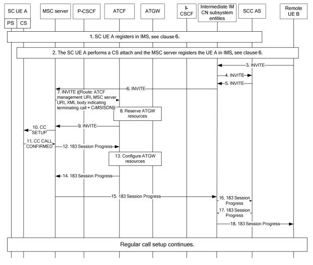
NOTE: For clarity, the SIP 100 (Trying) responses are not shown in the signalling flow.
