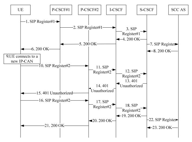
Figure A.3.2-1 Signalling flows for multiple registrations
