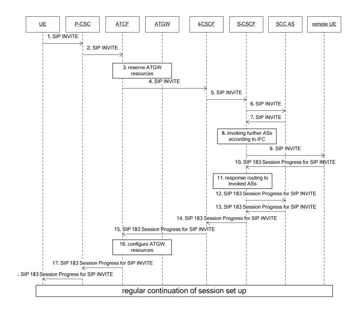
Figure A.4.2-1 Signalling flows for service continuity using PS to CS SRVCC enhancements
