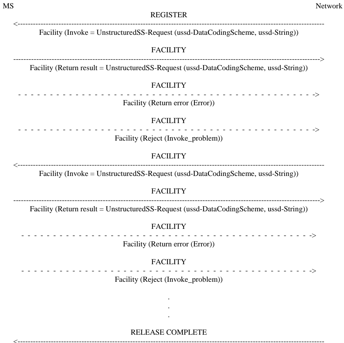
Figure 5.2: Multiple network initiated USSD request
