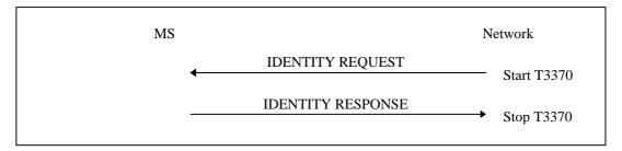
Figure 4.7.8/1 3GPP TS 24.008: Identification procedure
