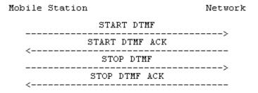
Figure 5.8/3GPP TS 24.008 Single DTMF transmission
