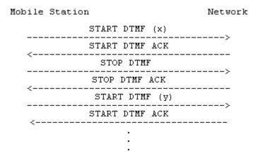
Figure 5.9/3GPP TS 24.008 Multiple DTMF transmission
