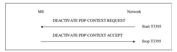
Figure 6.11/3GPP TS 24.008: MBMS context deactivation procedure
