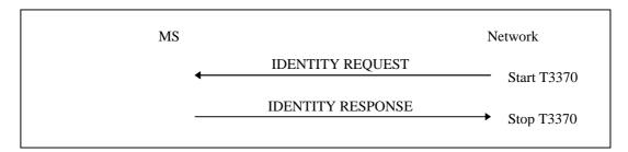
Figure 4.7.8/1 3GPP TS 24.008: Identification procedure
