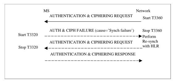
Figure 4.7.7b/1 3GPP TS 24.008: Authentication failure cause "Synch failure"
