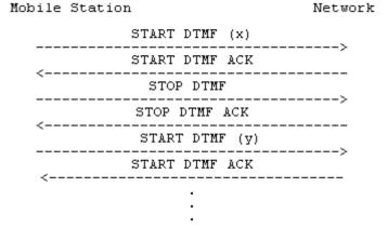
Figure 5.9/3GPP TS 24.008 Multiple DTMF transmission
