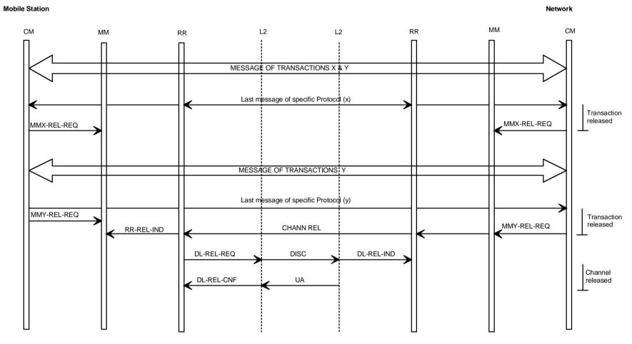
Figure A.7: Release of parallel transactions (General view)
