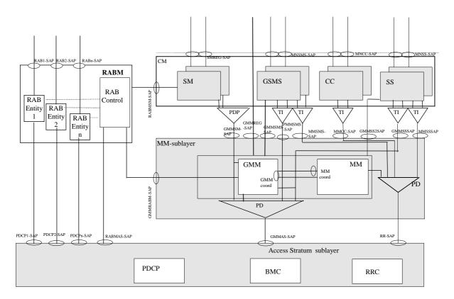
Figure 5.6/24.007: Protocol architecture of Non Access Stratum supporting CS/PS mode of operation MSs, MS – side
