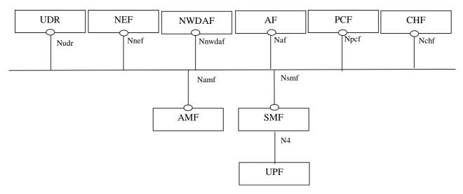
Figure 5.2.1-1: Overall non-roaming reference architecture of policy and charging control framework for the 5G System (service based representation)
