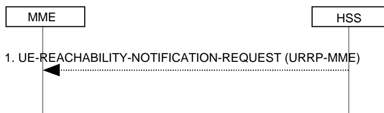
Figure 5.3.11.2-1: UE Reachability Notification Request Procedure
