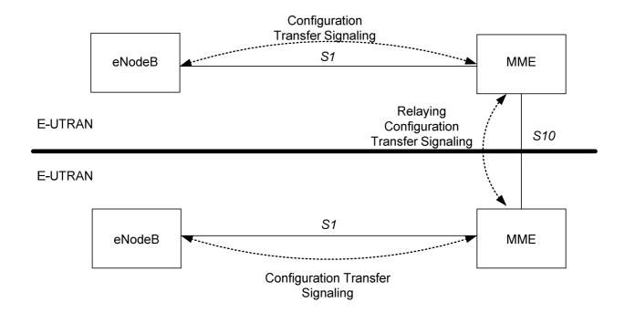
Figure 5.14-1: inter E-UTRAN Configuration Transfer basic network architecture
