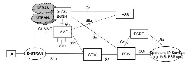
Figure D.2.2-1: Non-roaming Architecture for interoperation with Gn/Gp SGSNs
