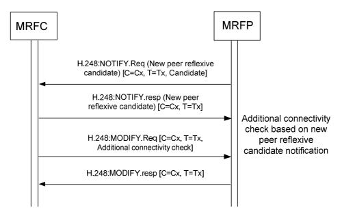
Figure 6.2.18.4.1: Procedure to perform additional connectivity check upon the report of new peer reflexive candidate
