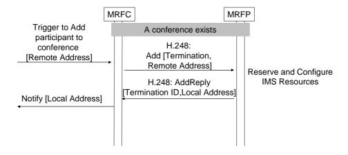
Figure 6.2.9.3 Procedure to add user in Dial-in scenario
