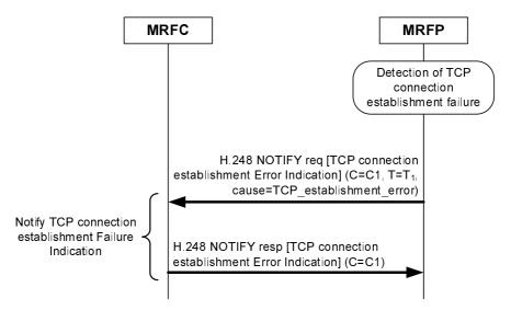
Figure 6.2.20.2.1: TCP connection establishment Failure Indication
