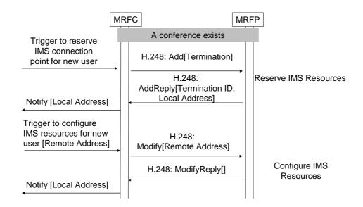
Figure 6.2.10.2 Procedure to add user in Dial-out scenario
