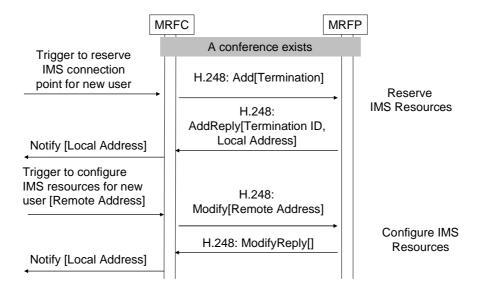
Figure 6.2.9.2 Procedure to add user in Dial-out scenario
