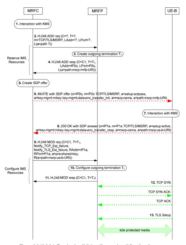
Figure 6.2.19.2.2.1: Terminating ("dial-out") example call flow for e2e case
