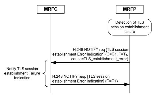
Figure 6.2.19.4.1: TLS session establishment Failure Indication
