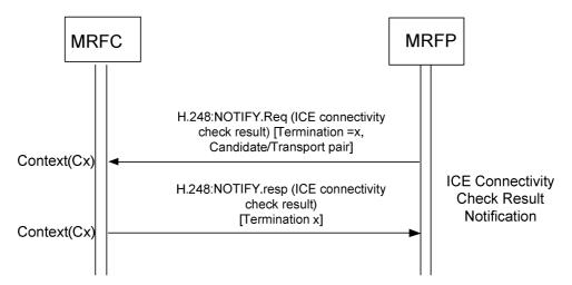
Figure 6.2.18.3.1: Procedure to report ICE connectivity check result
