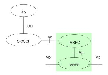
Figure 4.1: Architecture of MRF
