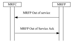
Figure 6.1.2.2: MRFP indicates the Failure/Maintenance locking
