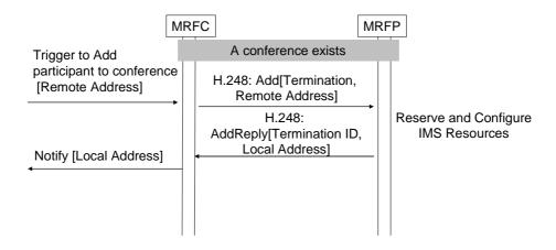
Figure 6.2.10.3 Procedure to add user in Dial-in scenario
