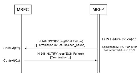
Figure 6.2.14.3.1: Procedure to Report ECN Failure
