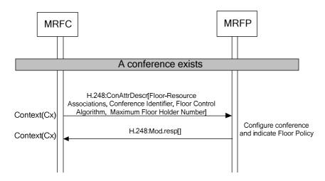
Figure 6.2.13.2.2.1 Procedure to Configure Conference for Floor Control
