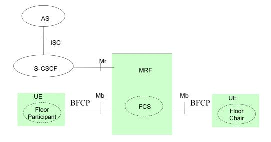
Figure 5.14.2.1: Functionality Architecture of Floor Control
