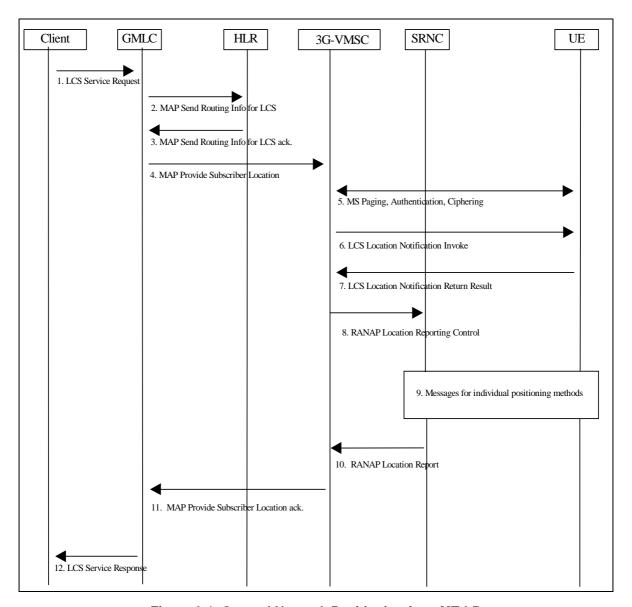
Figure 8.4: General Network Positioning for a MT-LR
