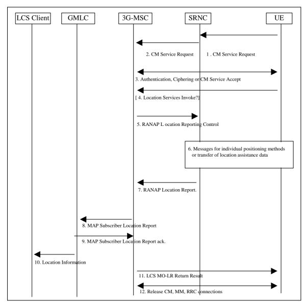
Figure 8.8: General Network Positioning for MO-LR
