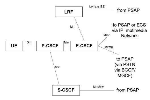
Figure 5.1: E-CSCF in reference architecture
