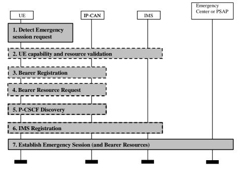
Figure 7.1: Terminal Detected Emergency Calls
