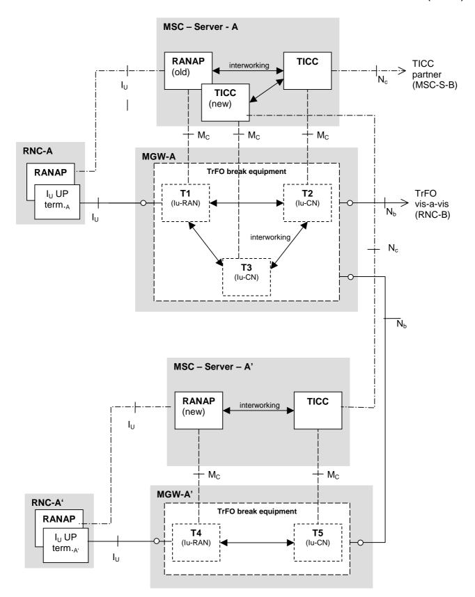
Figure 6.2/4: Configuration during inter-MSC SRNS Relocation
