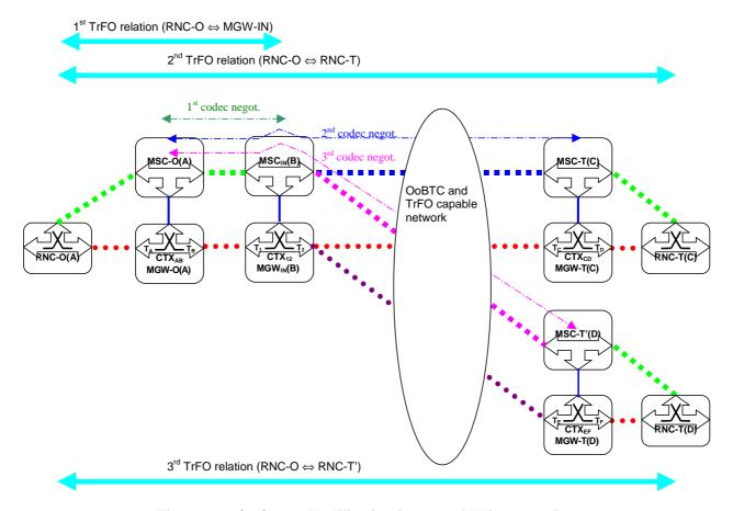
Figure 6.3.2/1. Codec Modification in case of IN interworking
