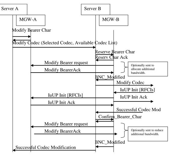
Figure 5.8.4/1: Successful Codec Modification including luFP
