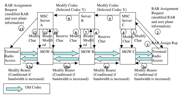
Figure 5.8.1/1: Codec Modification Control Procedures
