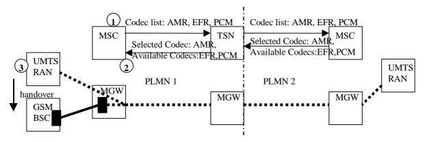
Figure 6.5/1: UMTS to GSM Inter-System Handover
