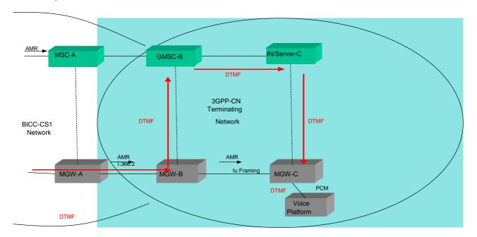
Figure 5.9/1:DTMF received inband from external network
