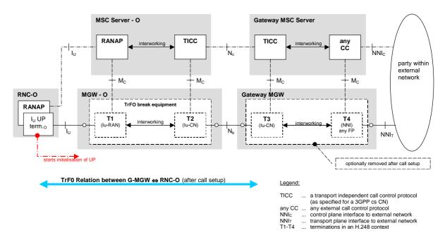
Figure 6.8/1. Configuration during Call Setup of a Mobile to External Network Call
