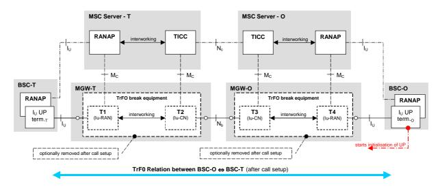
Figure 6.9/1: Configuration during Call Setup of a Mobile to Mobile Call for GERAN lu-mode
