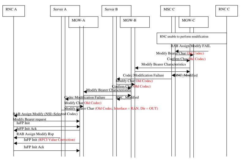
Figure 5.8.5/2: Call Sequence for Unsuccessful Modification. Call Flow Part 2
