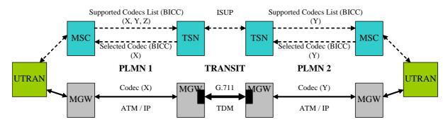
Figure 5.5/1: Cascaded TrFO & Transcoding
