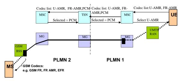
Figure 5.5/2: UMTS to GSM interworking
