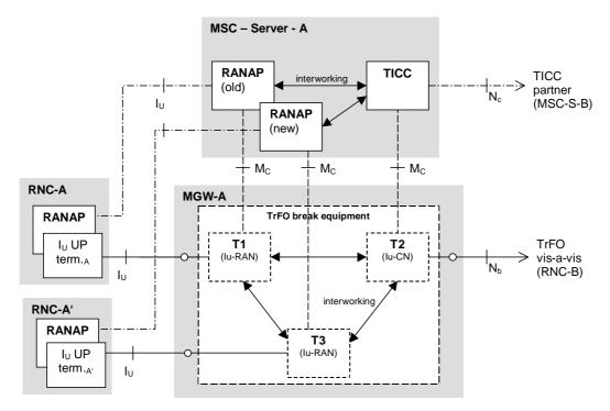
Figure 6.2/1: Configuration during intra-MSC SRNS Relocation
