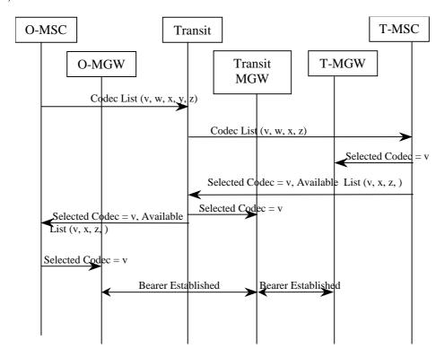
Figure 5.2/1. Basic Codec Negotiation Sequence
