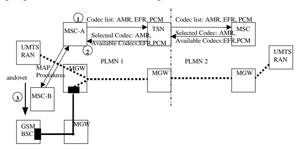
Figure 6.5/2: Inter-MSC, UMTS to GSM handover
