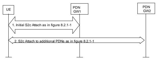
Figure 8.2.9-1: UE-Initiated connectivity to additional PDN from Trusted Non-3GPP IP Access with DSMIPv6 on S2c
