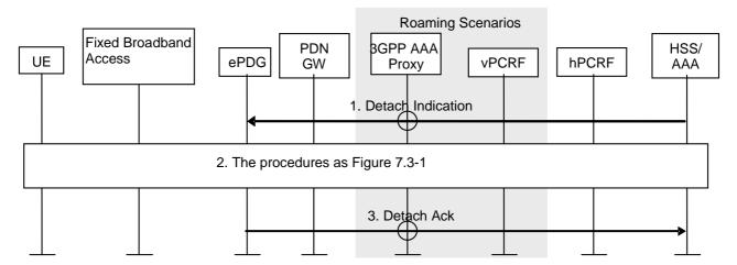
Figure 7.4-1: HSS/AAA-initiated detach procedure
