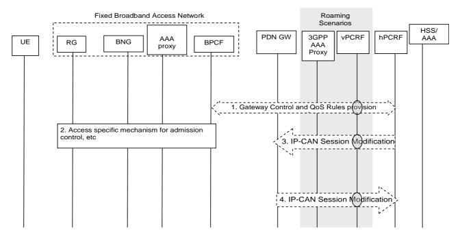
Figure 8.2.7-1: Network-initiated dynamic policy control procedure in Trusted BBF IP Access for DSMIPv6 on S2c
