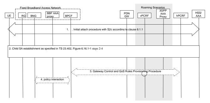
Figure 8.2.10-1 Activation of enhanced security for S2c
