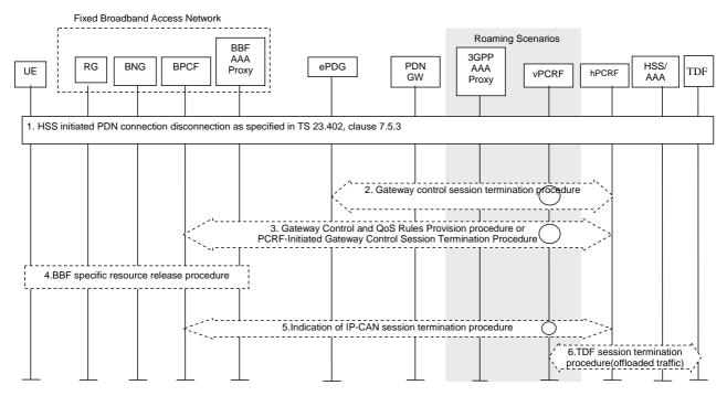
Figure 8.3.3-1: HSS-initiated detach procedure with DSMIPv6 on untrusted s2c
