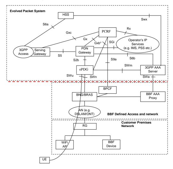
Figure 4.2.2-1: Non-Roaming Architecture for untrusted Fixed Broadband access network based on S2h
