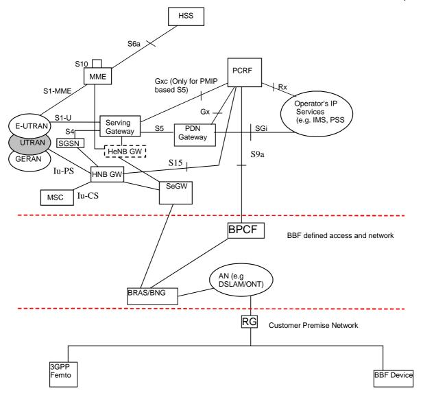
Figure 4.3.2-1: Non-Roaming Architecture
