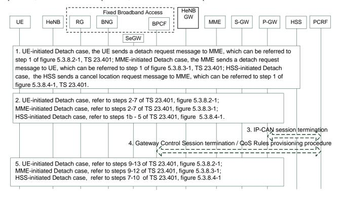
Figure 9.1.2: Detach Procedure via HeNB- UE camping on E-UTRAN
