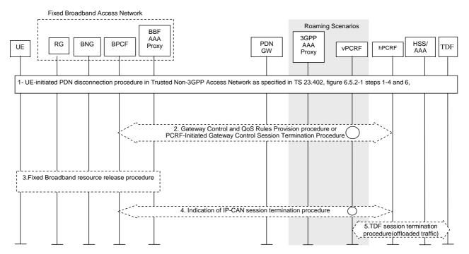
Figure 8.2.2-1: UE-initiated detach procedure with DSMIPv6 on trusted s2c
