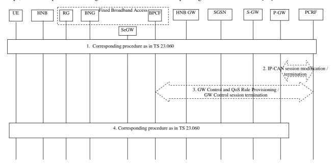
Figure 9.3.3-1: PDP Context/Bearer Deactivation Procedure for EPS-connected 3G access
