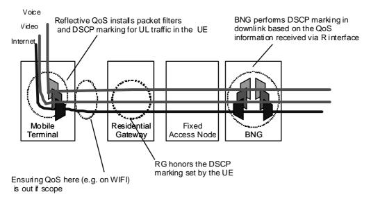
Figure 6.3.1-2: Packet classification and packet forwarding treatment in a 3GPP-Fixed Broadband Access interworking scenario for NS-WLAN offload traffic
