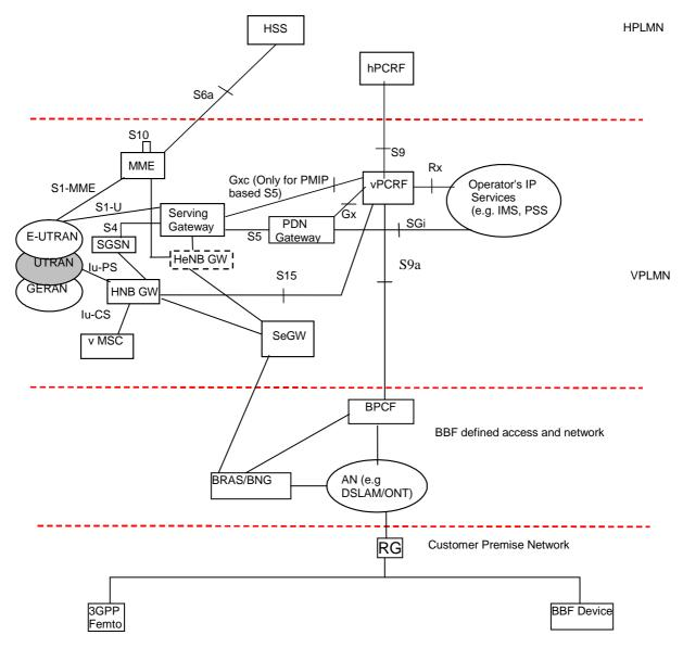
Figure 4.3.4-1: Roaming Architecture - Visited Access/ Local Breakout
