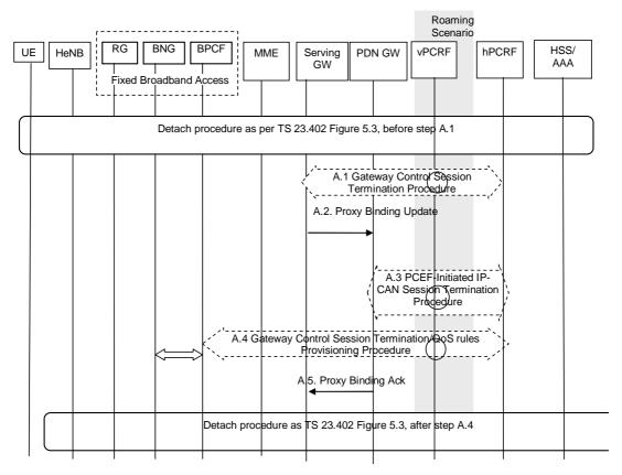
Figure 9.2.2-1: E-UTRAN Detach Procedure for PMIP-based S5/S8
