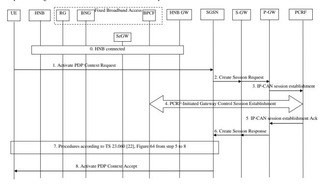
Figure 9.3.1-1: PDP Context Activation Procedure for EPS-connected 3G access
