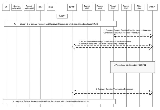
Figure 9.2.8-1: Service Request and Handover Procedures-S5/S8 PMIP-based
