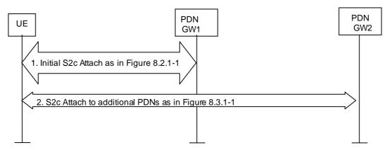
Figure 8.3.9-1: UE-Initiated connectivity to additional PDN from untrusted Non-3GPP IP Access with DSMIPv6 on S2c
