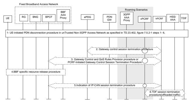
Figure 8.3.2-1: UE-initiated detach procedure with DSMIPv6 on untrusted S2c
