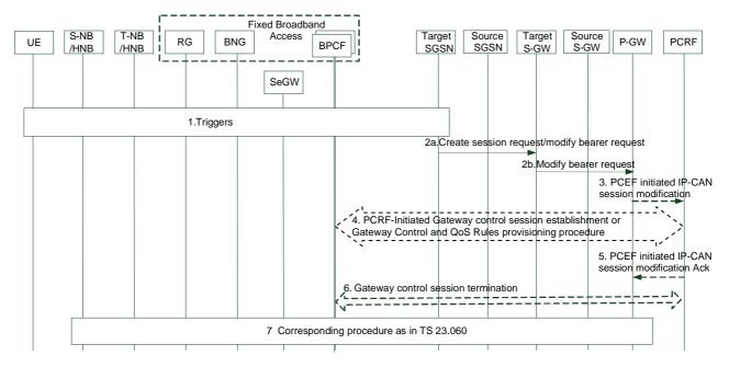
Figure 9.3.4-1: Service Request and Handover Procedures for EPS-connected 3G access
