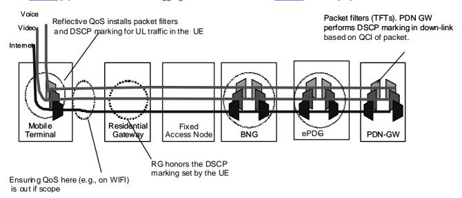
Figure 6.3.1-1: Packet classification and packet forwarding treatment in a 3GPP-Fixed Broadband Access interworking scenario for traffic routed to EPC
