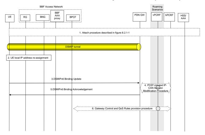
Figure 8.2.11-1: UE local IP address changes on S2c over trusted Fixed Broadband Access
