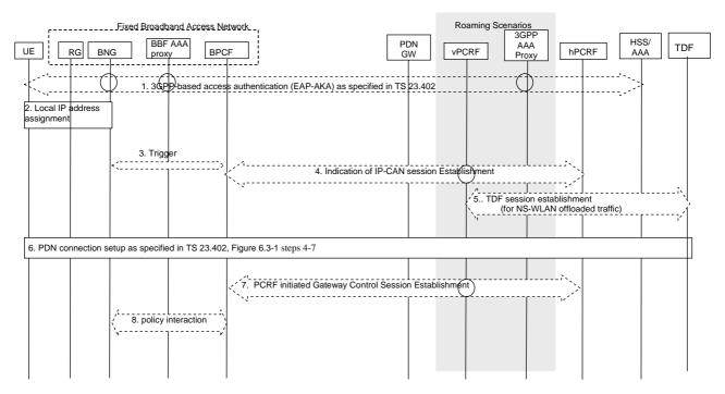
Figure 8.2.1-1: Initial attachment with DSMIPv6 when S2c is used for roaming, non-roaming and LBO
