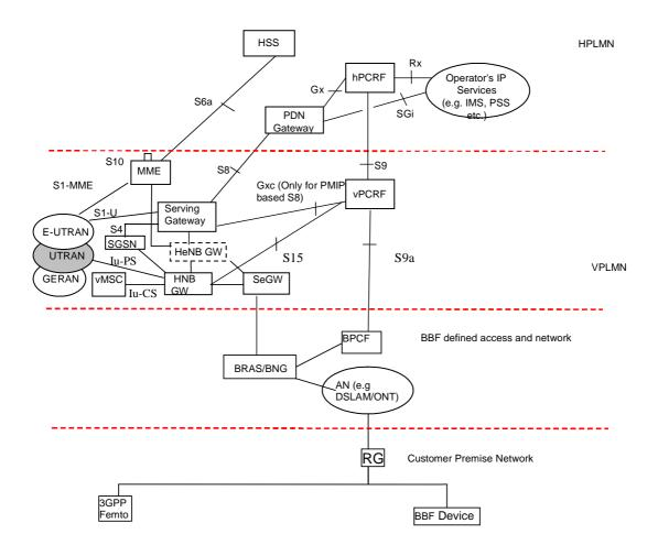
Figure 4.3.3-1: Roaming Architecture - Home Routed Traffic
