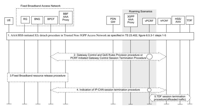
Figure 8.2.3-1: HSS-initiated detach procedure with DSMIPv6 on trusted s2c
