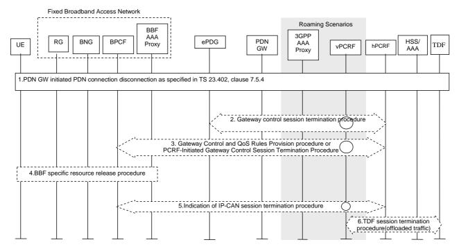
Figure 8.3.4-1: PDN GW-initiated PDN disconnection procedure with DSMIPv6 on untrusted s2c
