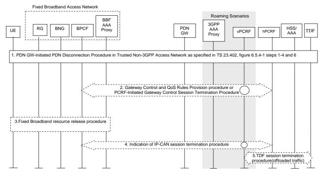
Figure 8.2.4-1: PDN GW-initiated PDN disconnection procedure with DSMIPv6 on trusted S2c
