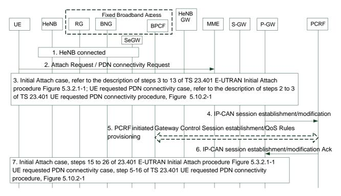
Figure 9.1.1: UE Attach and UE requested PDN connection Establishment procedure via HeNB
