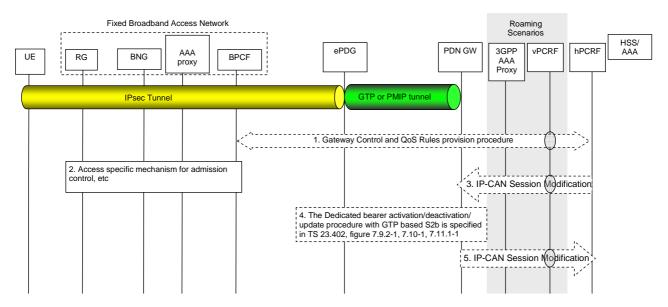
Figure 7.6-1: Network-initiated dynamic policy control procedure
