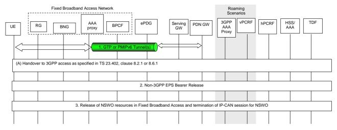
Figure 7.10-1: Handover from Fixed Broadband Access to 3GPP Access
